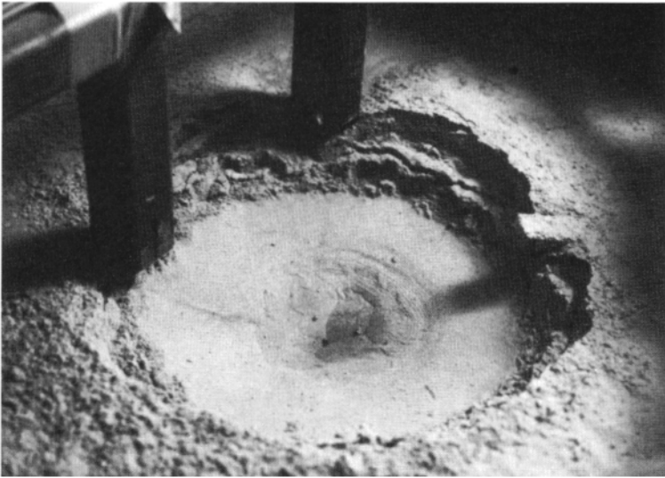
Figure 7.14 Crater formation from a buried blast at 60 g in saturated sand.
