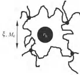
Figure 1.7 The effects of molecular size ( r_h ) on the diffusion of a solute in a network of pore size \xi
