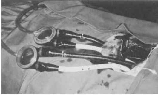
Figure 5.6 The MEDOS HIA ventricular assist device (The picture shows a configuration that was used in animal experiments at the Groningen University, The Netherlands)
