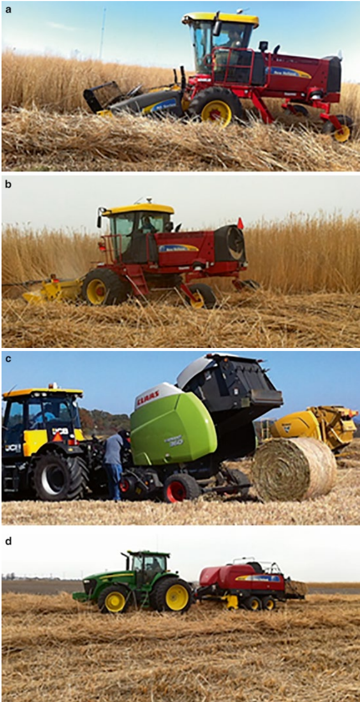
Fig. 5.24 Harvesting machinery for energy grasses: (a) a sickle head mower-conditioner mowing switchgrass, (b) a rotary disk head mower-conditioner mowing Miscanthus, (c) a large round baler baling switchgrass, and (d) a large square baler baling Miscanthus
