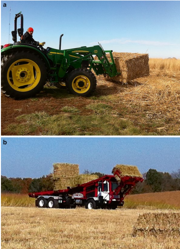
Fig. 5.22 (a) Tractor-mounted front loader to pick up and transport large square bales. (b) A self-propelled automatic bale loading machine
