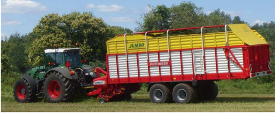
Fig. 5.19 Self-loading wagon (Pöttinger Jumbo 8000). Adapted from [23]
