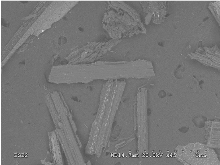
Fig. 2.2 Cross-sectional surface of switchgrass ground particles under scanning electron microscope
