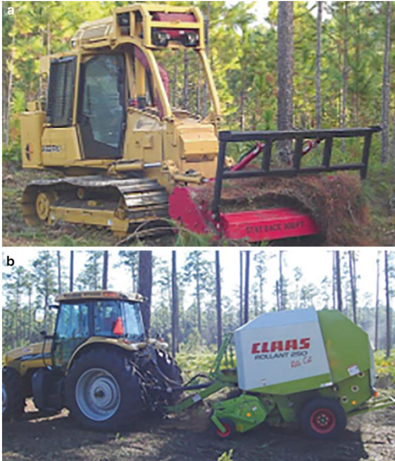
Fig. 5.28 (a) BH-120 Fecon head mulcher. (b) Claas Rollant 250 round baler used to harvest forest understory bushes. Adapted from [25]
