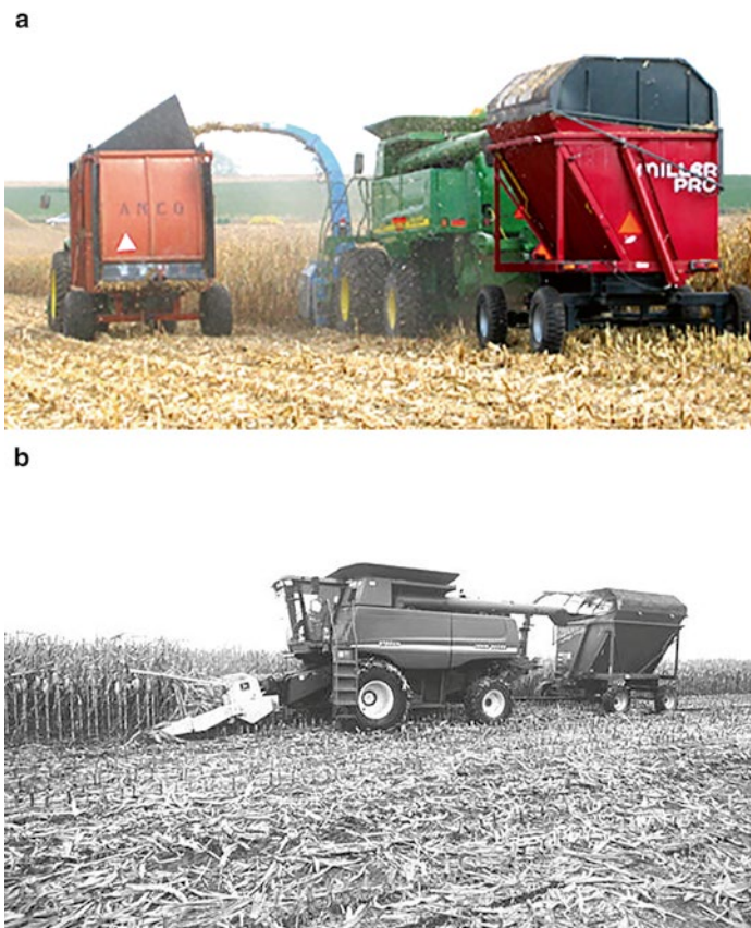
Fig. 5.37 Single-pass corn stover and grain harvester. (a) Grain combine modified with a stalk-gathering head (front) and cob-gathering head (back). (b) A grain combine modified with a whole-plant head and gathering cobs and husk. Adapted from [33]
