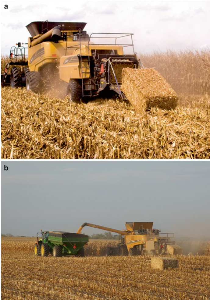
Fig. 5.38 Combine-baler systems. (a) AGCO-developed combine-baler baling corn stover. Photo courtesy of AGCO Corporation [34]. (b) Single-pass machine showing grain harvest and corn stover baling. Photo courtesy of Dr. Matthew Darr, Iowa State University [35]
