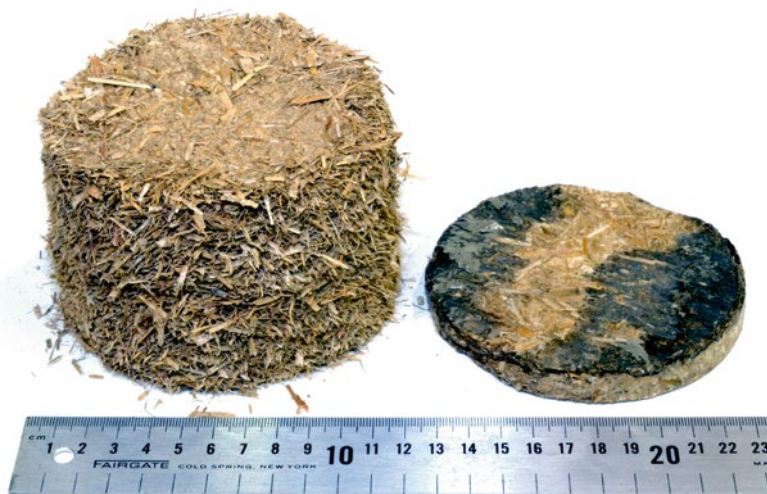
Fig. 6.4 Left : sample of Miscanthus ground to 12.7-mm particle size at a density of 350 \text{ kg m}^{-3} . Right : sample after being exposed to a pressure of over 750 MPa at a density of approximately 1,470 \text{ kg m}^{-3}
