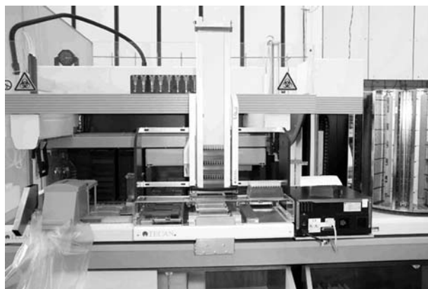
Fig. 2.10 Pipette robot Genesis (Tecan GmbH, Maennedorf, Switzerland) with integrated carousel (right) [5 h].
