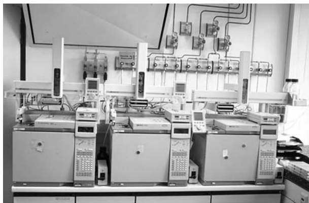
Fig. 2.17 Picture of optimized unit for ee -determination based on three gas chromatography instruments driven by one PC [26c].
