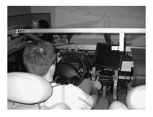
FIGURE 22.10 Subject operating a radio while driving in a vehicle simulator.
