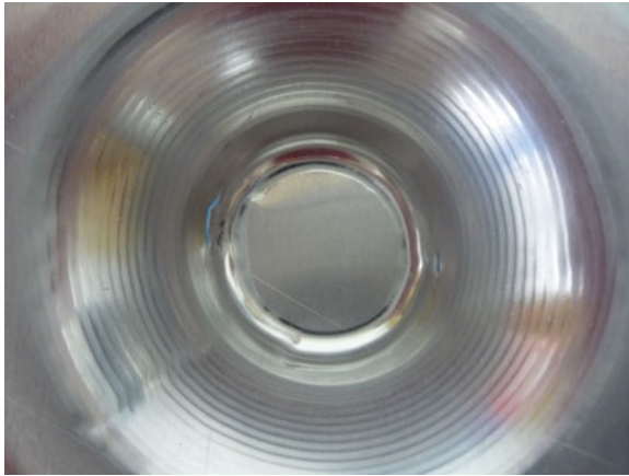
Fig. 16 Photo of the formed part with changed tool path and crack propagation ( I test)
