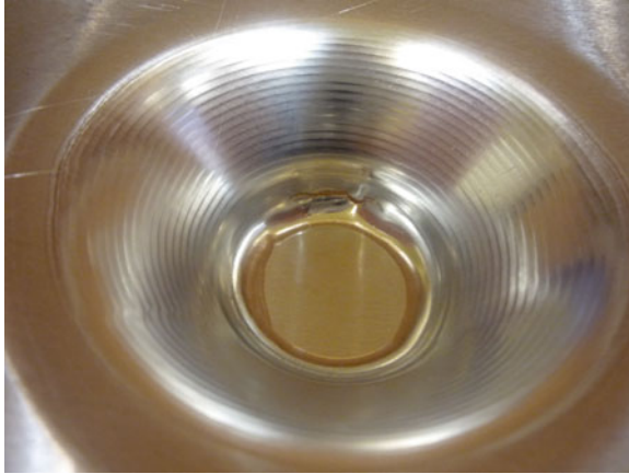
Fig. 22 Photo of the formed part with changed tool path and crack propagation (3 test)
