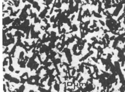
Fig. 2: Ni-Cu- $\text{Al}_2\text{O}_3$  composite (hot-pressed, electroless plated alumina particles first by Cu and then by Ni, porosity ~2%) dark areas alumina particles.
