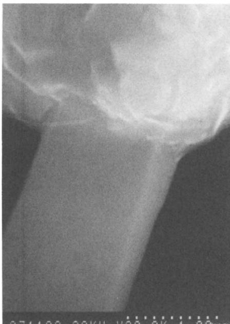
Figure 4. SEM micrograph of  $\beta'$ -sialon whisker with polycrystalline root.
