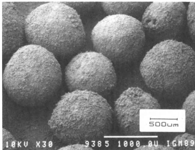
**Fig. 9 - Iron-Coated WC-Co particles.**
