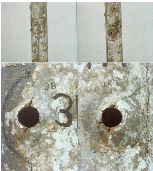
Fig. 4.1—Bullet-perforated casing from a surface test.
