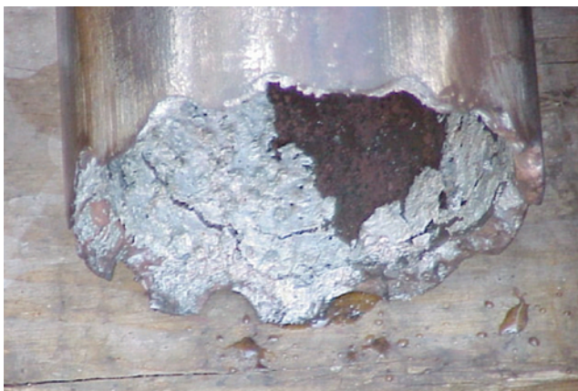
Fig. 4.16—Cut produced by a thermite cutter.
