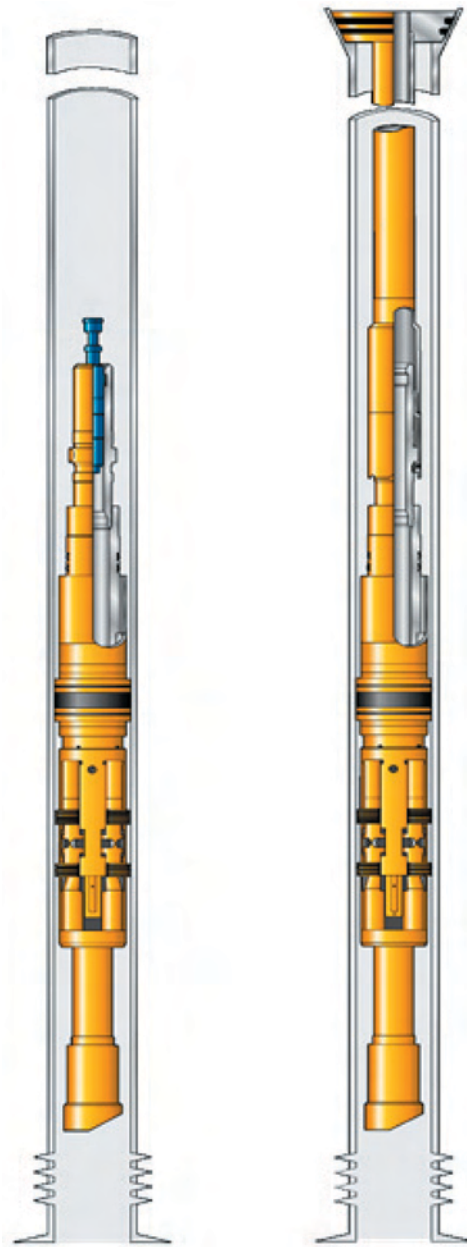
Fig. 2.4—Wireline-set tubing retrievable packer. Shown set with plug in place (first view) and with tubing connected and plug retrieved (second view).
