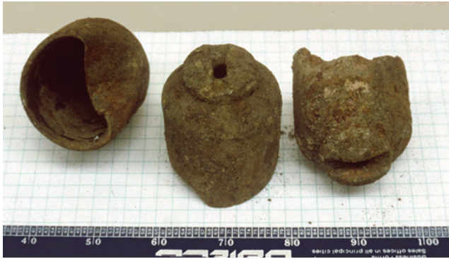
Fig. 4.6—Charge cases removed from a low-order gun.
