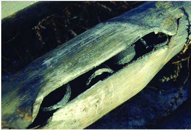
Fig. 4.7—Burst gun fished from a well after low-order firing.
