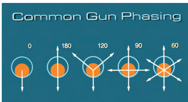
Fig. 4.8—Common perforator phasing.
