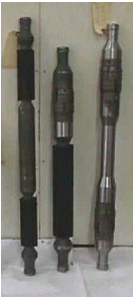
Fig. 16.26—Pad/brush combination plungers (left to right): brush/brush, brush/pad, pad/pad configurations. (Courtesy of Ferguson Beauregard.)
