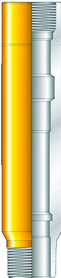
Fig. 2.17—Selective profile nipple.
