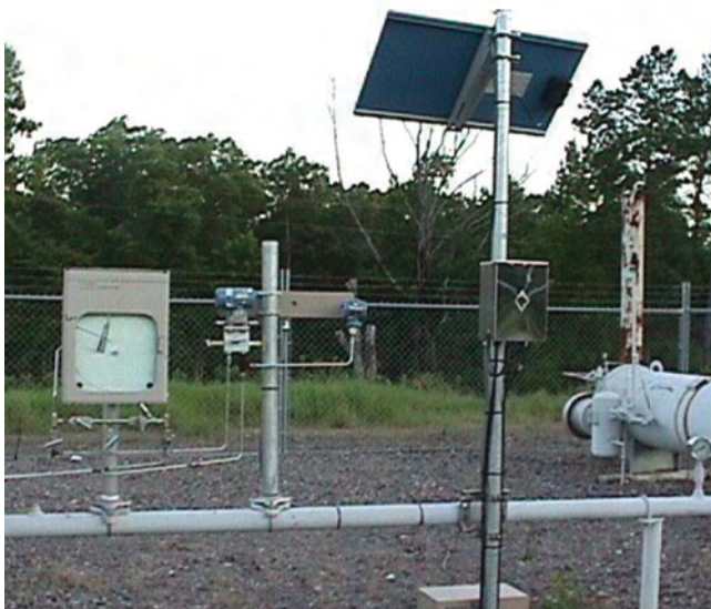
Fig. 16.34—Plunger-lift controller that incorporates electronic gas measurement and telemetry. (Courtesy of Ferguson Beauregard.)
