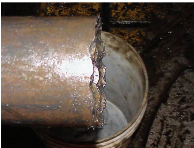
Fig. 4.14—Chemical cut pipe.
