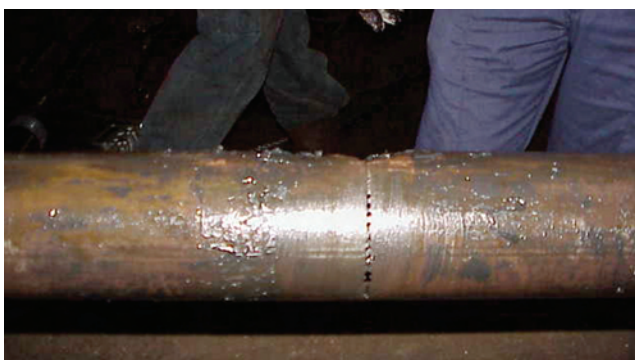
Fig. 4.15—Partial chemical cut.
