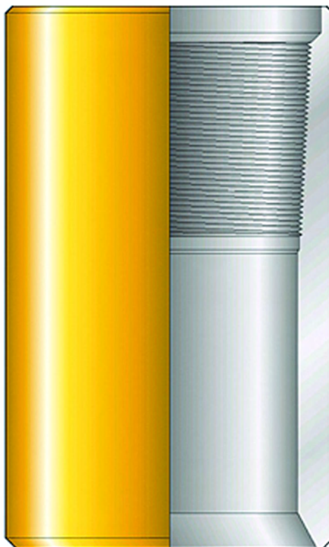
Fig. 2.14—Wireline re-entry guide.
