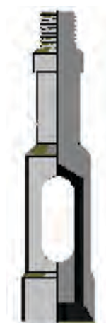
Fig. 16.15—Cutaway of a gauge ring. (Courtesy of Ferguson Beauregard.)
