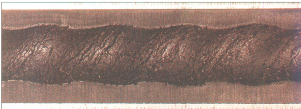
Fig. 15.45—High-temperature stator damage.
