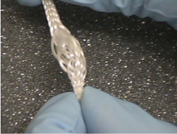
Fig. 3.3 A photograph of a poly lactide, three-dimensional 5 \times 5 square braid developed for ligament regeneration research in an in vivo rabbit model study; open structure substitute for intra-articular anterior cruciate ligament and tighter braided edge region for bone tunnel fixation
