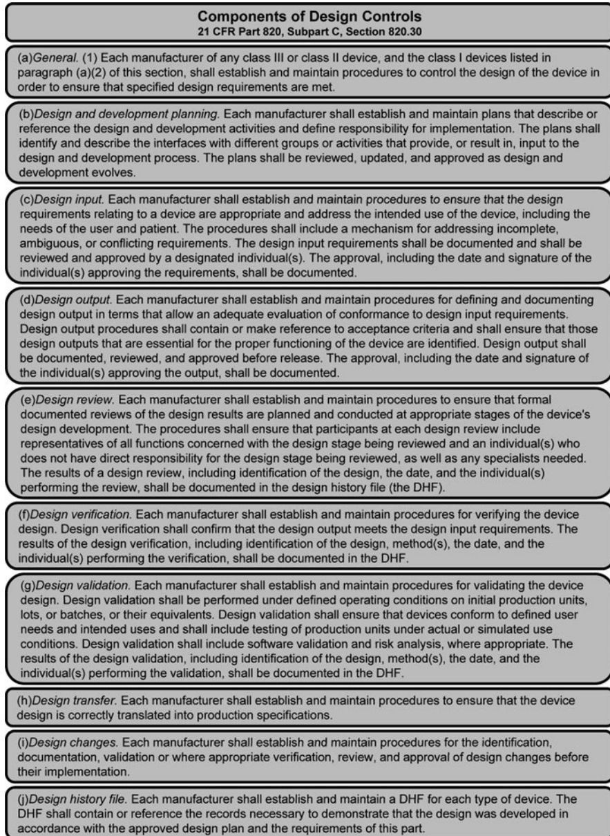
Fig. 19.2 Summary of the components of the design control framework. Source: 21 CFR Part 820, Subpart C, Section 820.30
