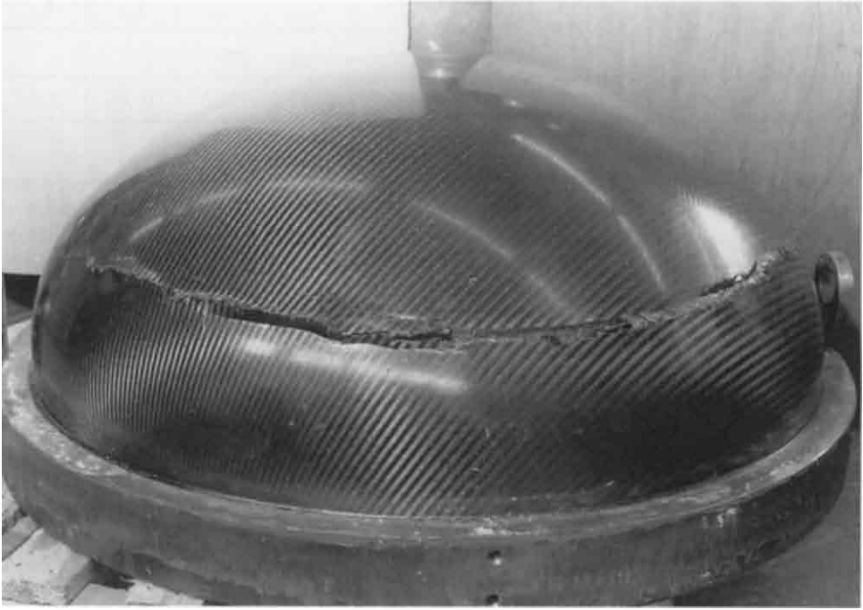
Fig. 2 30-ply CFRP torisphere after a failure test
