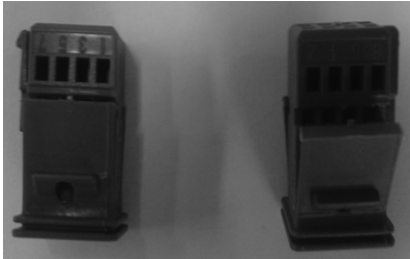
Figure 3. 8-pole plastic connector – a front view.
