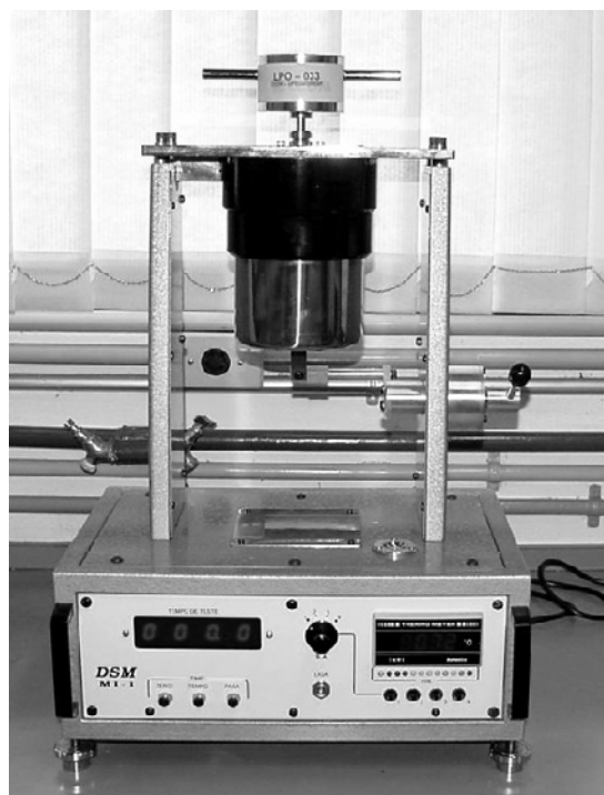
Fig. 1 MFI equipment test
