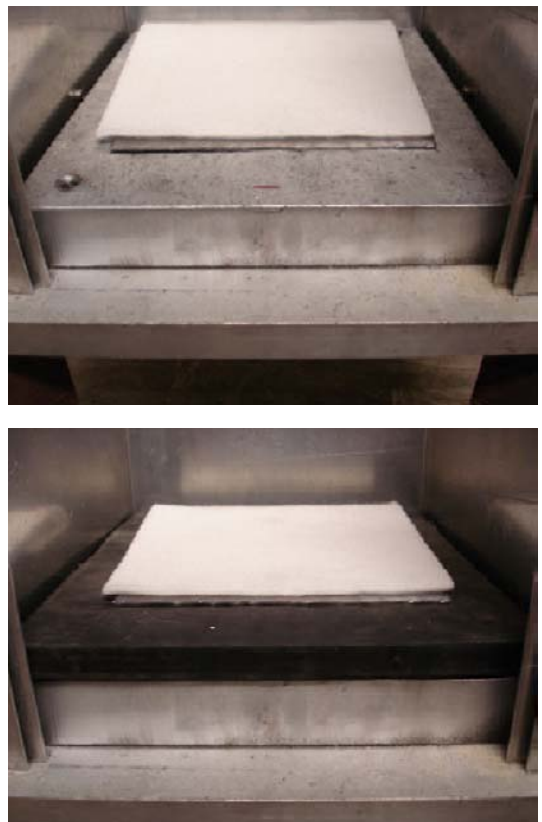
Fig. 3 Rigid and deformable support configurations
