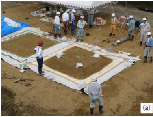
Fig. 8 Pictures of the field test: (a) hybrid geosynthetics, (b) HDPE geomembrane was installed
