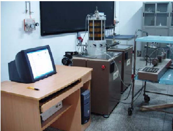
Fig. 1 GDS two-way dynamic triaxial testing system
