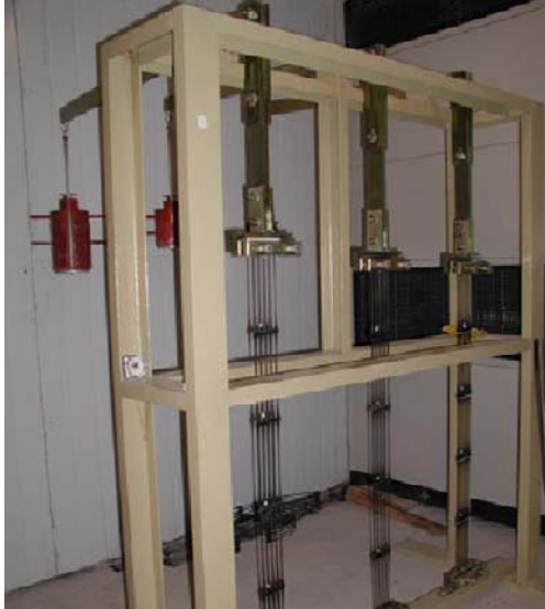
Fig. 1 Creep test facility
