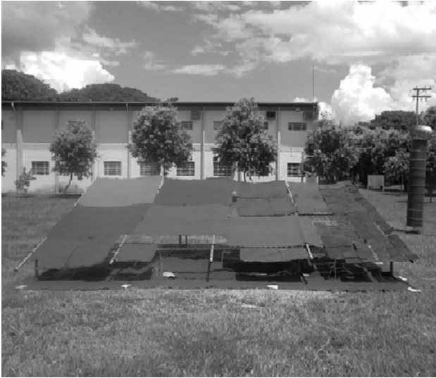
Fig. 2 Geotextiles samples exposed to weathering
