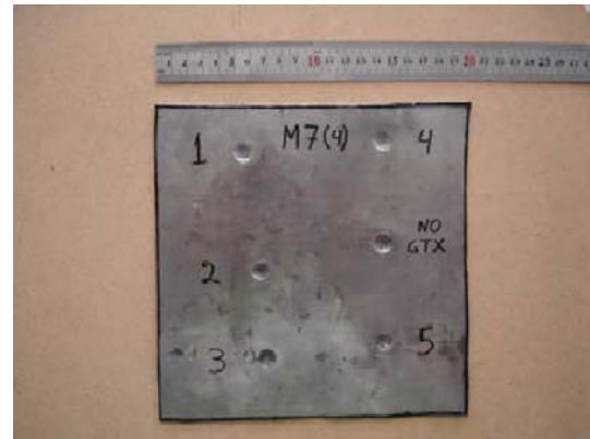
Fig. 4 Typical impacted lead plate
