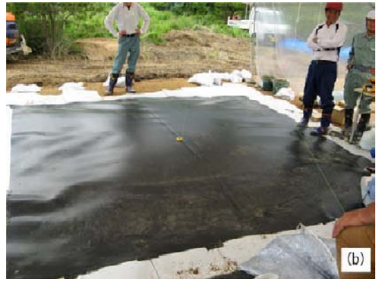
Fig. 8 Pictures of the field test: (a) hybrid geosynthetics, (b) HDPE geomembrane was installed
