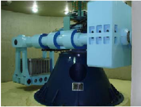
Fig. 1 Geotechnical centrifuge machine
