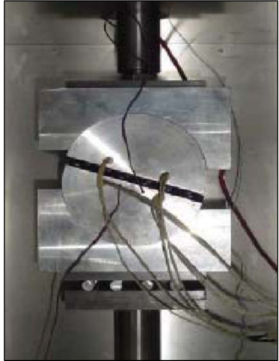
Fig. 6 TRI compression SIM incline test
