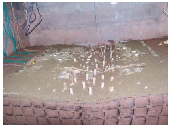
Fig. 7 Test model No. 4 deformation and failure of reinforced cushion
