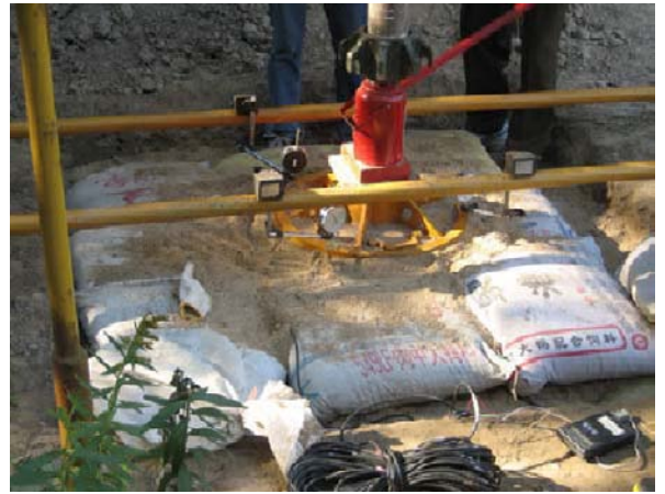
Fig. 4 Plate Load tests on soilbag reinforced foundation
