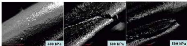
Fig. 9 Microscopic morphologies of Sample C after the test for various normal pressures
