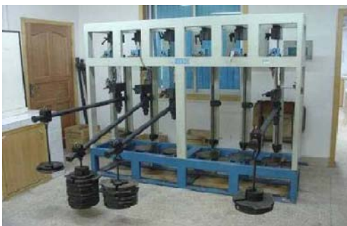
Fig. 1 Geo-synthetic materials and soil long-term deformation tester
