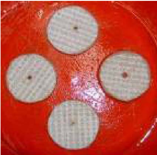
Fig. 2 Samples with different sizes of flaw
