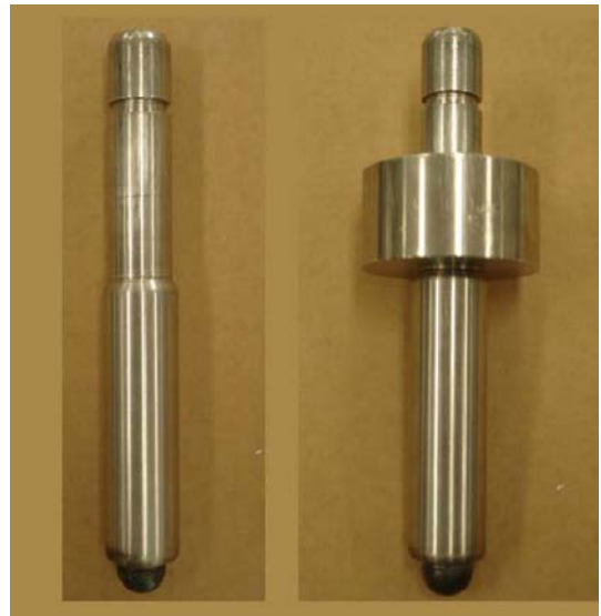
Fig. 2 Rigid probes, 1000g and 2000g mass
