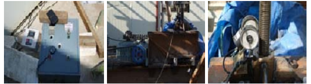
(a) control box (b) load delivery system (c) displacement measuring gauge
