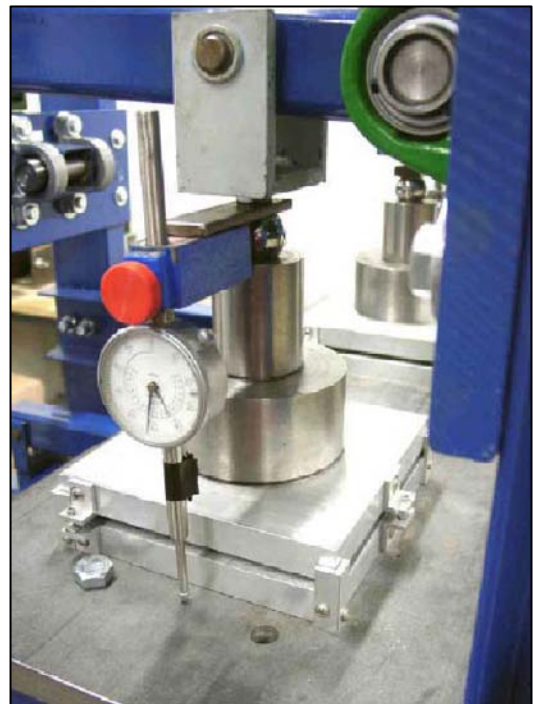
Fig. 5 TRI laboratory compression creep test
