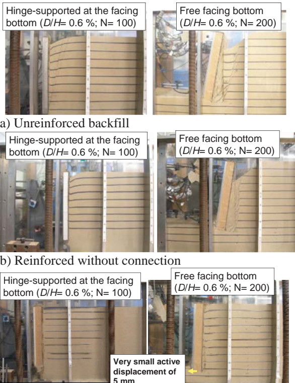
Fig. 13 Failure of backfill by cyclic active horizontal displacement of facing
