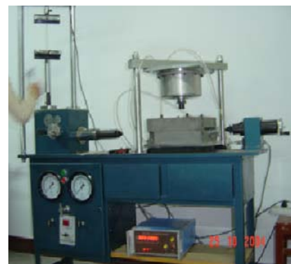
Fig. 3 Tensile test of the GFRP anchor
