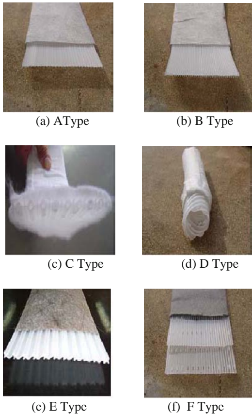
Fig. 2 Core Shape of Vertical Drain
