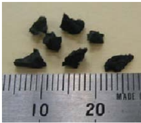
Fig. 2 Tire chips (Average diameter is 2 mm)
