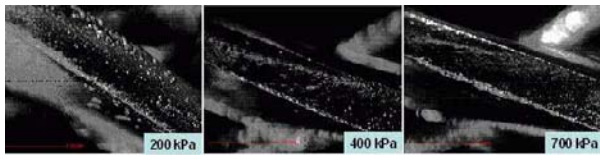
Fig. 7 Microscopic morphologies of Sample A after the test for various normal pressures
