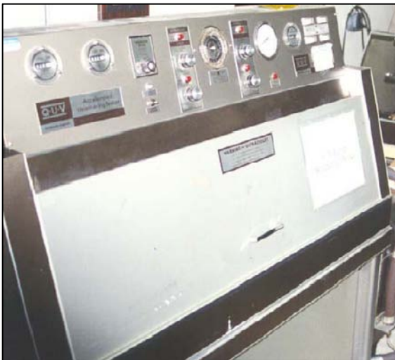
Fig. 2 Fluorescent UV weatherometers
