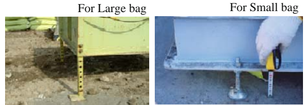
Fig. 2 Specification of filler volume ( Adjust the height of filling mould )
