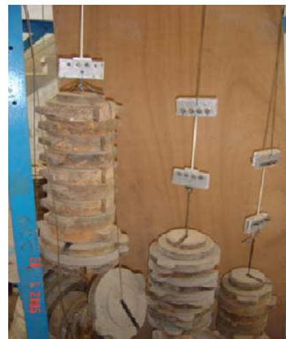
Fig. 4 Creep test of the GFRP anchor
