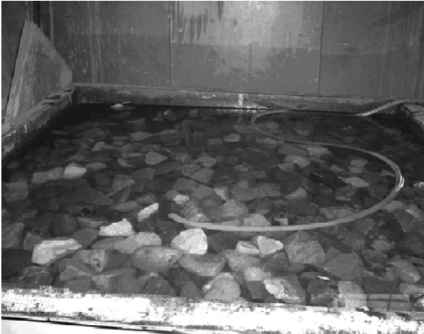
Fig. 6 Ballast in the saturated condition
