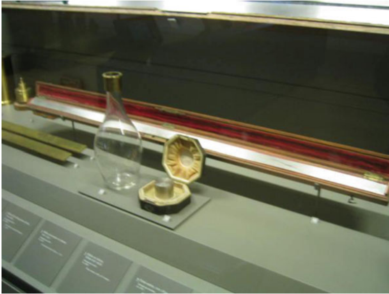
Fig. 2.16 Photo of platinum bar representing the meter in the Musée des Artes et Metiers, Paris
