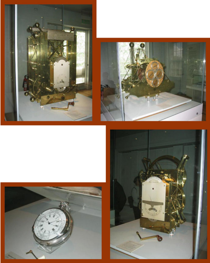
Fig. 2.15 Photos of John Harrison’s chronometers, numbers one through four clockwise from top left
