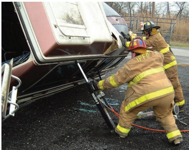
FIGURE 2-1 Ram used to right a rolled-over vehicle. (Courtesy of Mark Silverberg, MD.)
