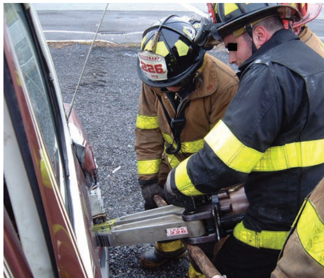
FIGURE 2-4 Jaws of life used to “pop open” a door to extricate a patient. (Courtesy of Mark Silverberg, MD.)
