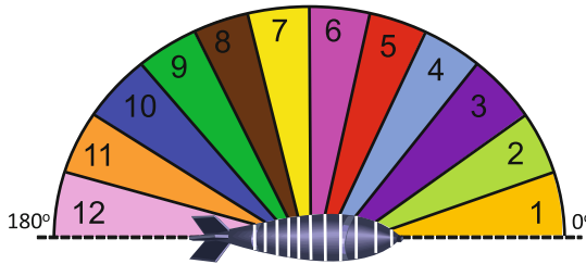
Fig. 2 The distributions of fragment numbers, masses and static ejection speeds from an exploding munition are dependent on the polar angle or zone, as measured from the nose (axially symmetric). In this example, the polar zones are numbered from 1 to 12
