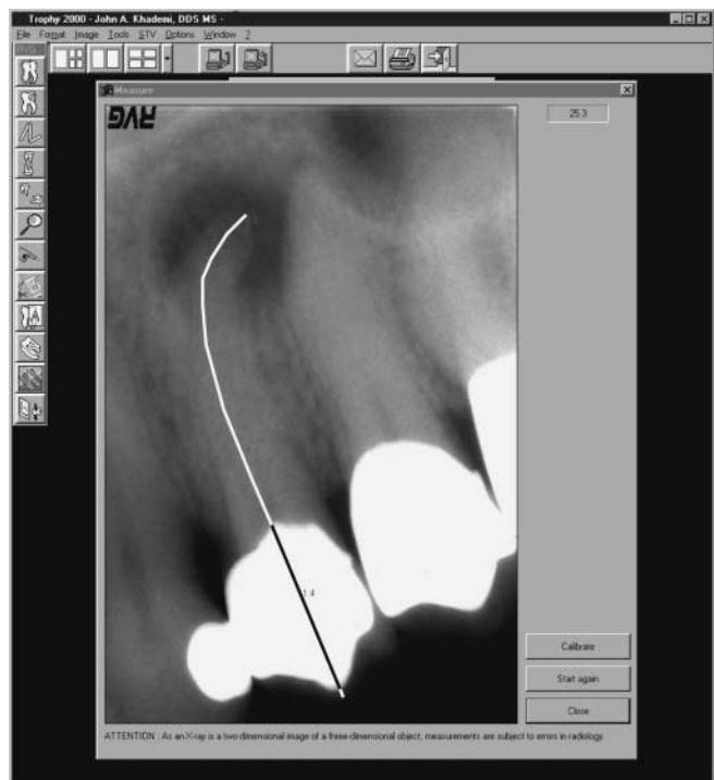
Figure 9-31 By beginning at the apex and advancing the cursor toward the crown with the "mouse," the computer will accurately calculate the working length of the tooth in millimeters, even around curvatures. (Courtesy of John A. Khademi.)
