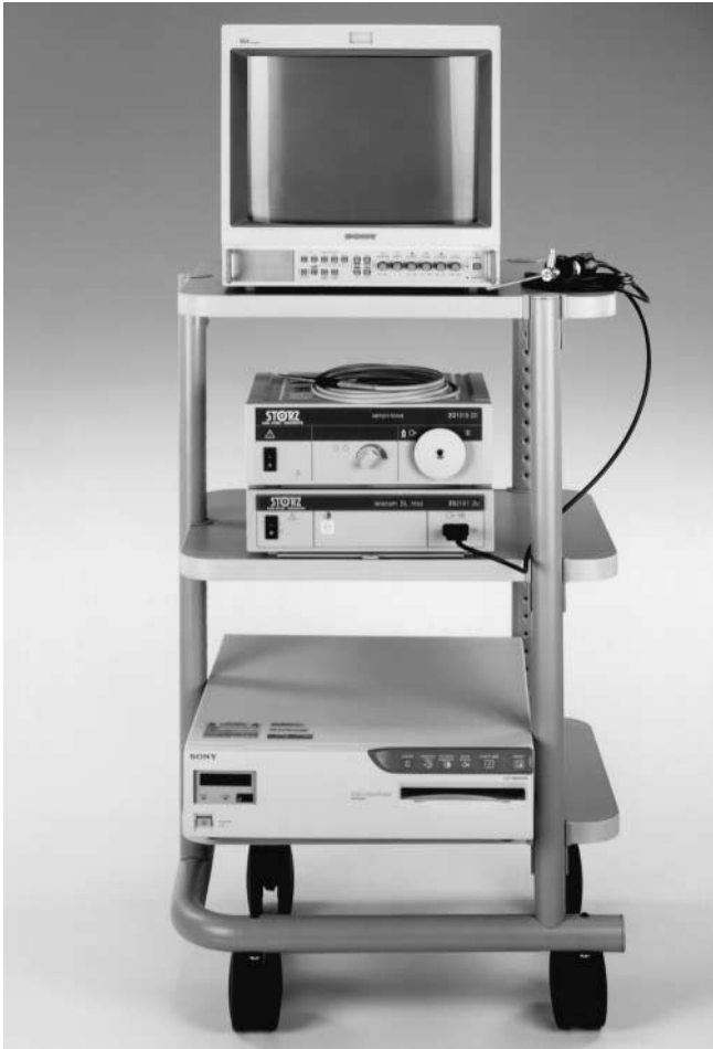
Figure 9-34 Endoscope set-up on mobile cart. Top shelf, Monitor, and to the right, camera head with scope attached. Middle shelf, Xenon light source on top of Telecam, the camera control unit, which is the heart of the system attached by cable to the camera scope above. Bottom shelf, Color printer. (Courtesy of Karl Storz & Co. Germany/USA.)
