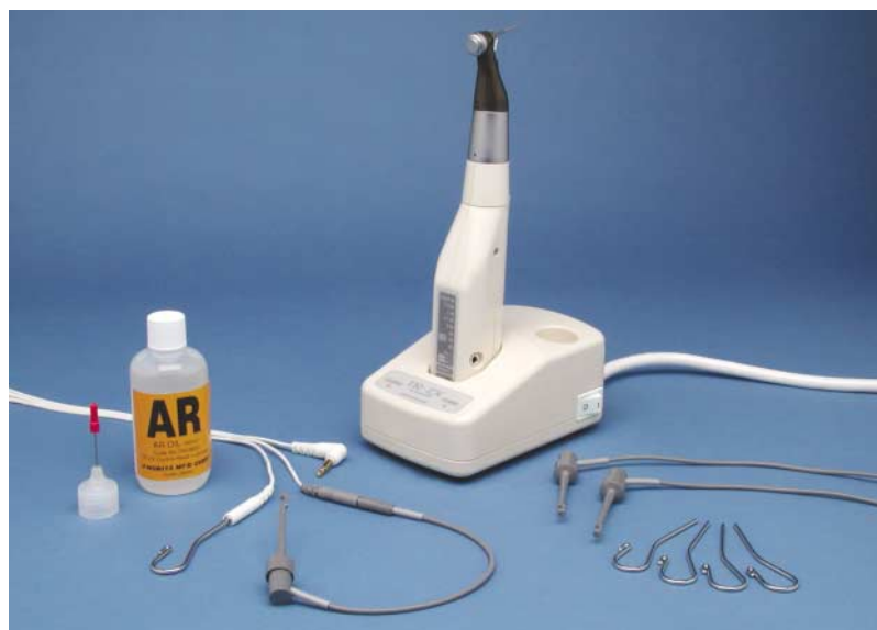
Figure 10-66 The Tri-Auto ZX is primarily a cordless, automatic, endodontic handpiece with a built-in Root ZX apex locator. The position of the nickel-titanium rotary instrument tip is constantly being monitored and displayed on the LED control panel. A built-in safety feature stops and reverses the motor when the apex is approached by the tip of the file. Accessories include (left) an AR contra-angle lubricant with a dispensing cap and apex locator attachments. Additional accessories (right). (Courtesy of J. Morita Mfg. Co.)
