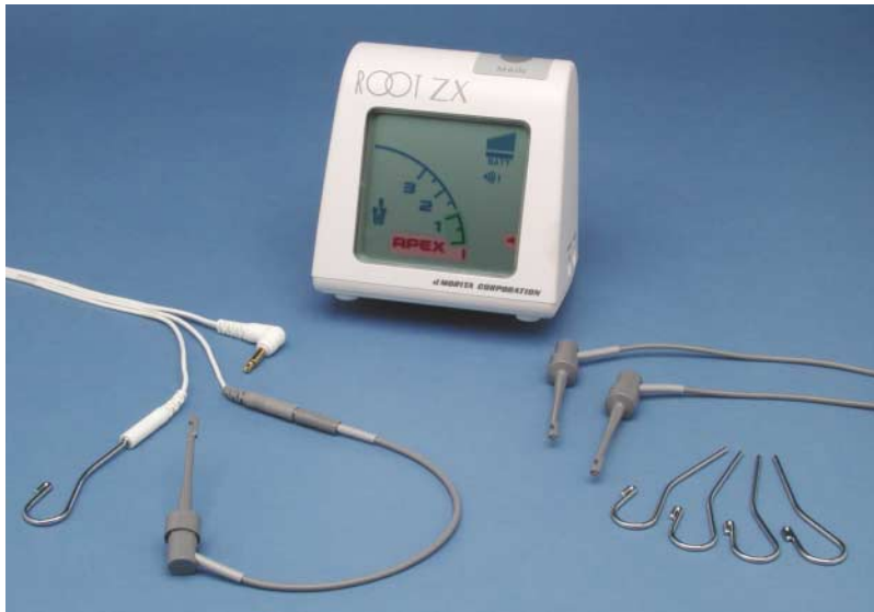
Figure 10-65 Root ZX third-generation apex locator with accessories (left) and extra accessories (right). The Root ZX microprocessor calculates the ratio of two impedances and displays a file's approach to the apex on a liquid crystal display. It functions in both a “dry” or canal “wet” with electrolyte. (Courtesy of J. Morita Mfg. Co.)
