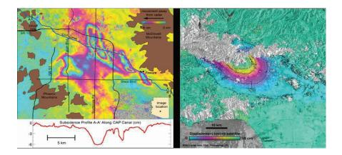
**FIGURE 3.6** Synthetic aperture radar interferograms. (a) Ground surface subsidence induced by changes in groundwater in Phoenix, Arizona (Tatlow and Buckley, 2003; used with permission). (b) Tectonic displacement field after the 1994 Northridge earthquake (image courtesy of Gilles Peltzer, University of California, Los Angeles; used with permission).
