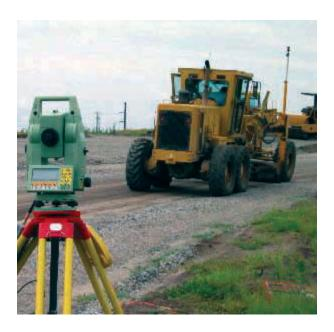
**FIGURE 2.4** Laser-guided earthmover (photo courtesy Lecia Geosystems, http://www.leica-geosystems.com).
