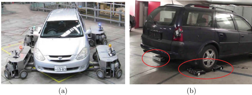
Fig. 2. (a) The iCART II robotic unit and (b) the next generation AVERT robotic solution, for extracting and carrying vehicles
