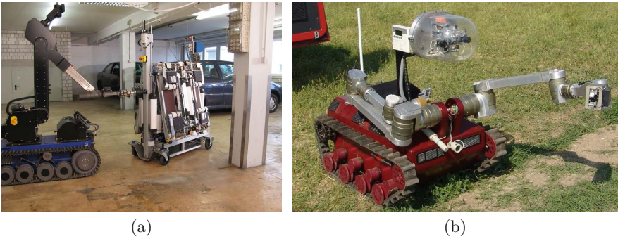
Fig. 3. (a) The police caterpillar robot, used for the neutralization of explosive mechanisms and (b) RESCUER robot operating in a field environment
