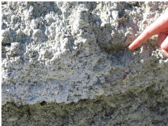
Fig. 7.6 Efflorescence of nesquehonite on the serpentinite tailing heap at Clinton Creek (Photograph by S.A. Wilson)
