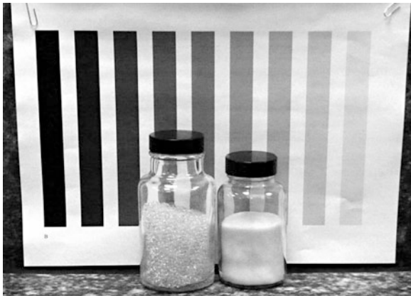
Fig. 4.5 The jar on the left contains 4 mm glass balls. The grey scale behind the jars has 10 bars going from roughly zero to nearly 100% whiteness depending on your printer and paper quality. This shows that the albedo of the 4 mm balls is about 0.6. The jar on the right contains 40 \mu\text{m} glass balls, 100 times smaller, and has an albedo of about 0.95
