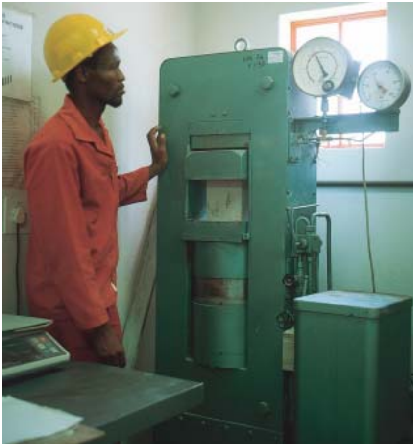
Figure 7: Daily testing of cubes ensures quality concrete
