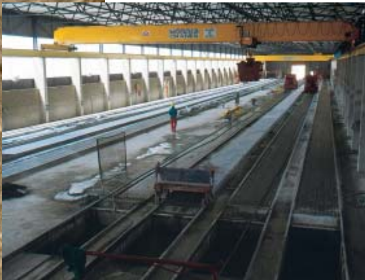
Figure 8: Manufacturing facility for prestressed hollow core slabs.
