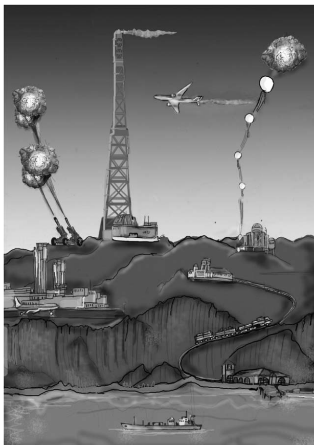
Figure 1 Proposed methods of stratospheric aerosol injection, including: airplanes, artillery, balloons and a tower. A mountain top location would require less energy for lofting to stratosphere. (Drawing by Brian West, Figure 1 from ref. 13).
