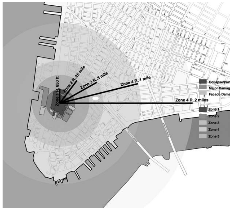
Figure 10.2 Assessment of the extent and type of damage. An area of 2 miles was affected.
