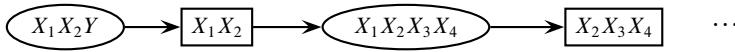
Fig. 5.4 A graphical illustration of the process of eliminating Y from \phi(X_1, X_2, Y) and X_1 from \phi(X_1, X_2, X_3, X_4) , where the ovals represent the domain of a potential before elimination and rectangles represent the domain of a potential after elimination
