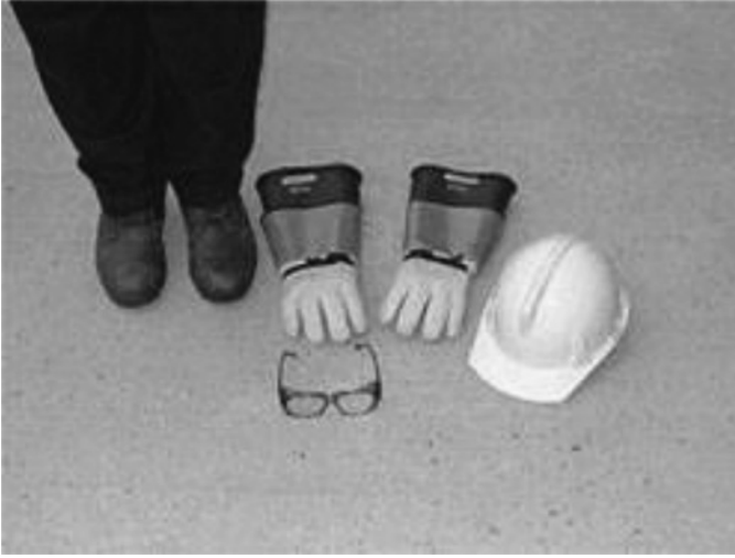
Figure 1.5 Photo of typical shock protection PPE. Source: Reproduced with permission of OSHA.
