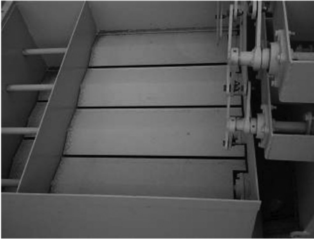
Figure 3.7 Secondary air damper before installation.
