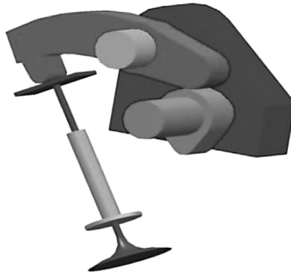
Figure 4.2 CAD model of the selected valve cam assembly.
