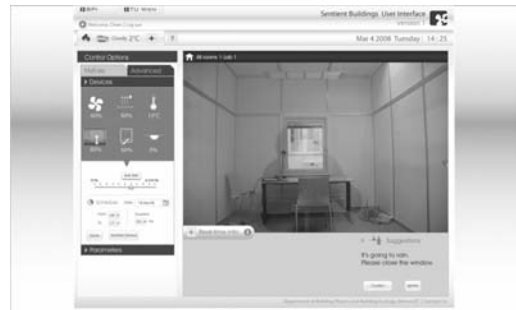
Figure 1. Sample screenshot of early interface prototype for test cells of the Building Automation Laboratory.
