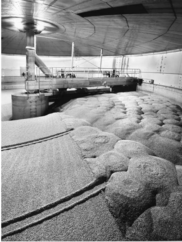
FIGURE 3.2 Flat-bottomed steeping vessel with automatic loading and unloading by radial dischargers. (Photograph courtesy of Bühler GmbH.)
