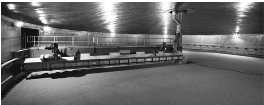
FIGURE 3.3 Circular single-floor kilning vessel. (Photograph courtesy of Bühler GmbH.)
