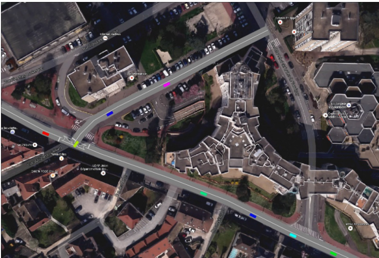
Figure 4.75. The model in simulation mode featuring four vehicles (green, blue, cyan, green) traveling south, three (green, blue, magenta) traveling east and one (red) arriving from the north. For a color version of this figure, see www.iste.co.uk/reveillac/modeling2.zip
