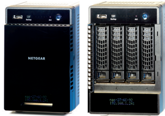
Netgear ReadyNAS 314: with front cover in place (left) and with front cover open (right).
