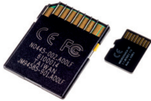
Comparison of SD and MicroSD cards
