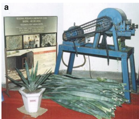
Fibre extraction using Raspador machine
