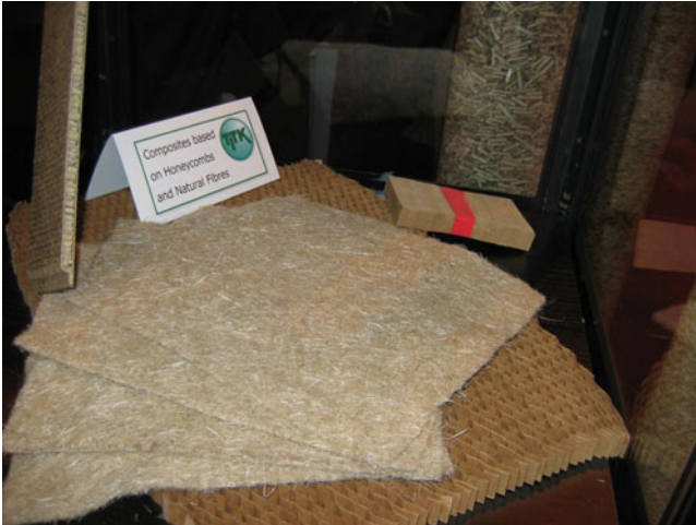
Fig. 23.10 Natural fibre skins for sandwich structures
