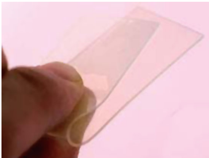
Fig. 21.10 Foldable transparent nanocomposites reinforced with bacterial cellulose nanofibers. Reproduced with permission from Nogi and Yano (2008). Copyright © 2008 Wiley-VCH Verlag GmbH & Co. KGaA, Weinheim
