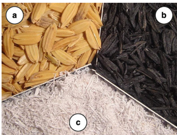
Fig. 13.2 Appearance of raw rice husks (a), black rice husk ash (b), and white rice husk ash (c)
