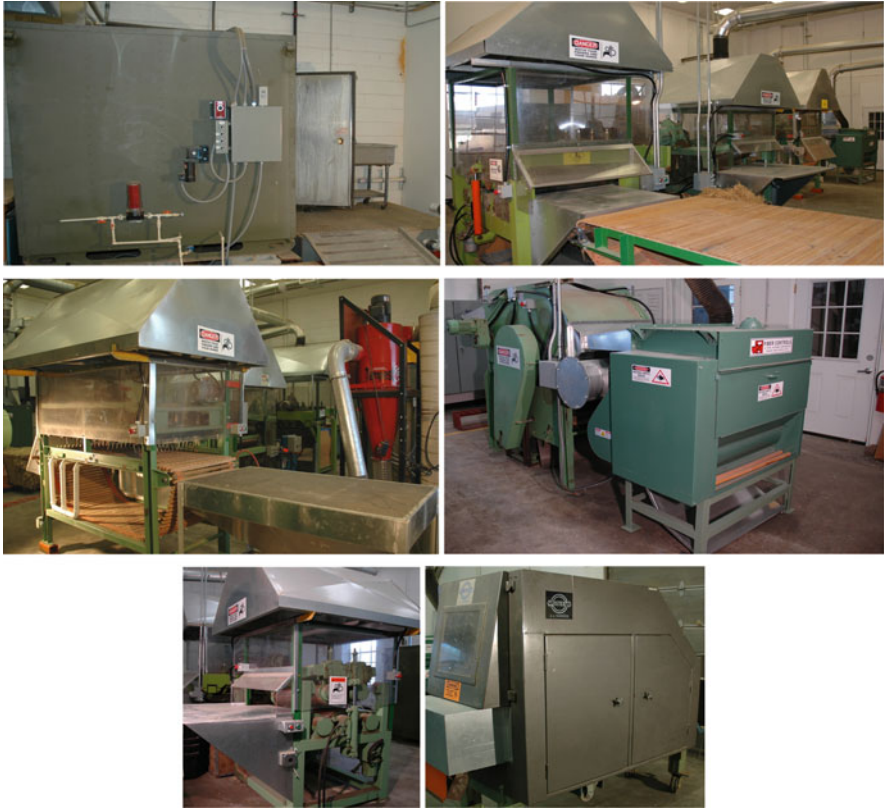
Fig. 3.1 Enzymatic-retting, washing, and drying system as part of the Flax-PP ( top left ). Nine-roller calendar for initial crushing and breaking of retted flax stems. Photograph showing view of entry point for flax between top four (3 grooved and 1 smooth) and five bottom rollers (two grooved and three smooth) ( top right ). Top shaker to remove shive from fiber ( middle left ). Scutching wheel that strokes flax to shorten and clean fibers with condenser for fiber collection after processing ( middle right ). Five-roller, grooved calendar with three bottom rollers and two top grooved rollers ( bottom left ). Flax Cottonizing Line guillotine chopper for cottonizing flax fibers as part of the Flax-PP ( bottom right )
