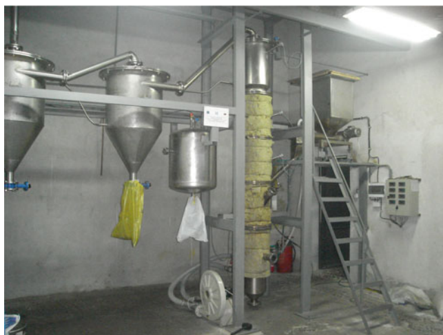
Fig. 13.6 A photograph of the pilot plant for rice husks pyrolysis
