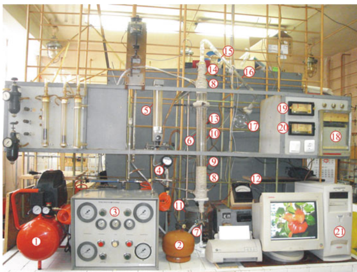
Fig. 13.5 A photograph of the laboratory equipment setup for combustion of raw rice husks in fluidized bed reactor (1) air compressor Black & Decker ; (2) tank for liquid petroleum gas (LPG); (3) distributor for gasses; (4) manometer; (5) air Rota meter; (6) quartz fluidized bed reactor; (7) gas burner; (8) asbestos insulator; (9) porous quartz diaphragm; (10) electrical heater; (11) electrical transformer; (12) voltmeter; (13–15) thermo couples; (16) economizer; (17) separator; (18) temperature recorder; (19, 20) thermo regulators; and (21) PC
