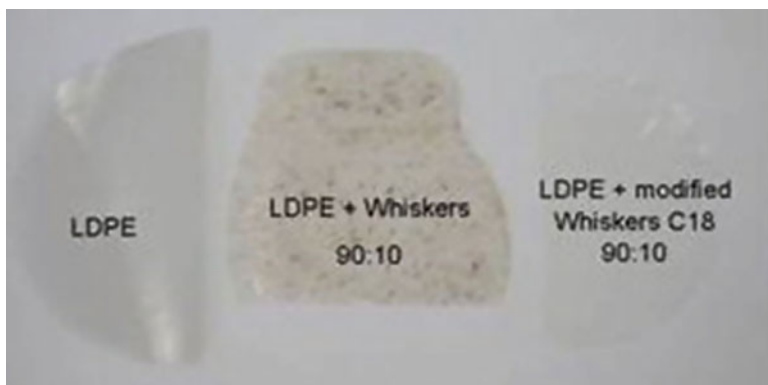
Fig. 7.4 Photographs of the neat LDPE film and extruded nanocomposite films reinforced with 10 wt% of unmodified and C18 acid chloride-grafted cellulose whiskers (de Menezes et al. 2009). Reproduced by permission of Elsevier
