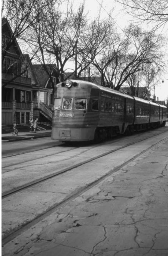
Figure 2.5: The Chicago, North Shore & Milwaukee was unusual among interurban electric railways in operating not only single cars but unitized trains, called Electroliners, articulated so they could negotiate the tight turns of the Loop in Chicago. In Milwaukee, they ran right through residential neighborhoods. The North Shore was one of the last interurbans to stay in business; after it was abandoned in 1963, the Electroliners got a second life with a line running between Philadelphia and Norristown. (Author's photo)
