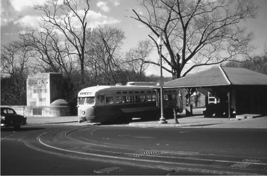
Figure 4.2: A postwar all-electric PCC with standee windows is seen here looping at the Calvert Street (now Duke Ellington) Bridge over Rock Creek. Washington, D.C.'s Capital Transit had one of the largest PCC fleets. (Author's photo)
