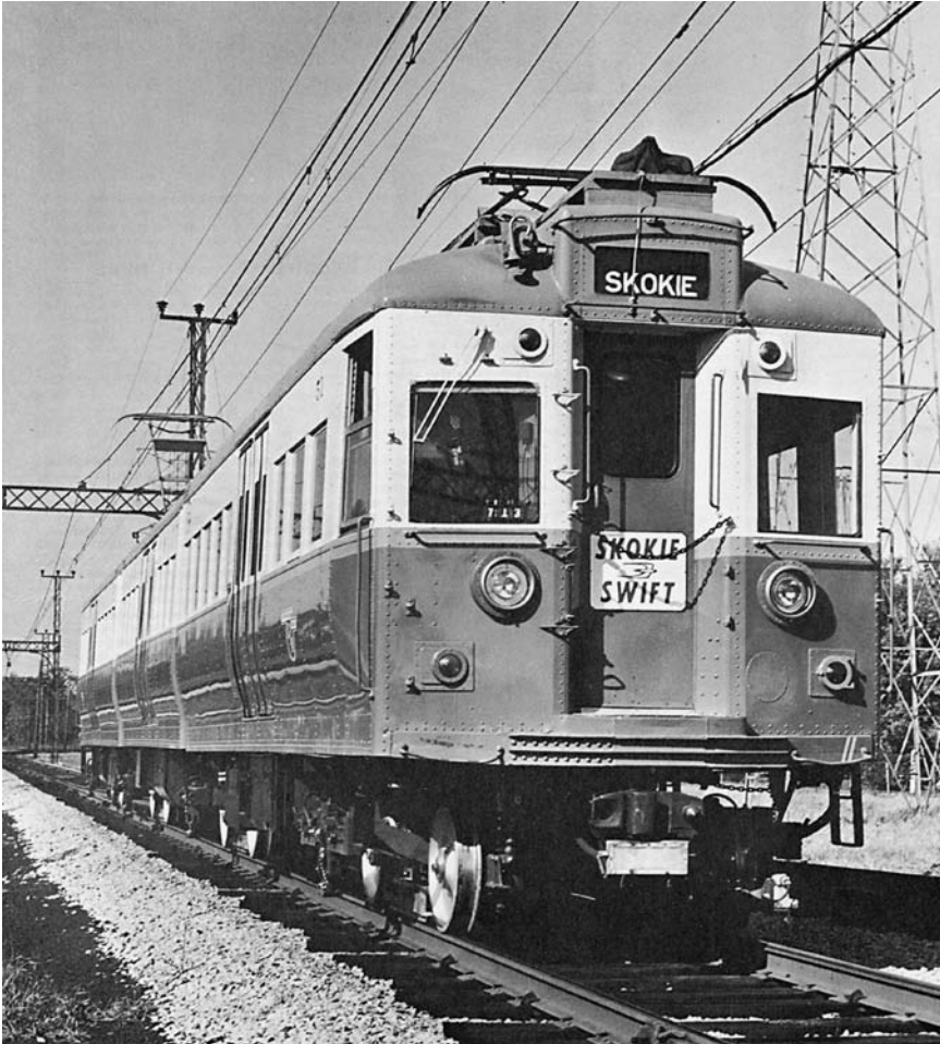
Figure 5.3: The Skokie Swift, which began operation in 1964, was light-rail transit before the name was invented. The cars were built using parts salvaged from PCCs and the line provided a connection between the Chicago Transit Authority's heavy-rail system in northern Cook County and the village of Skokie, near O'Hare Airport. (Chicago Transit Authority publicity photo, author's collection)
