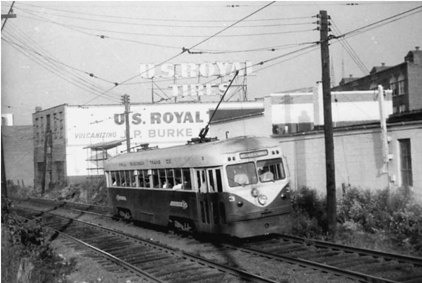
Figure 4.1: Brill’s answer to the PCC, a streamlined Brilliner, is seen here on private right-of-way on the western outskirts of Philadelphia. Brill had previously designed trolleys it dubbed Master Units whose “automotive styling” was carried over into Brilliners and then into rubber-tired transit vehicles. (Author’s photo)
