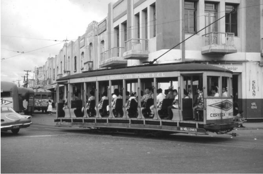
Figure 2.4: Open cars were boarded from the longitudinal step, from which the conductor also collected fares. This car, obtained second-hand from a Connecticut company by the Cooperativa de Transportes Urbanos y Sub Urbanos de Vera Cruz, operated year round. Cars similar to this one, but with a center aisle, were called “convertibles” and had side panels and windows that could be removed or replaced, depending on the season. (Author’s photo)
