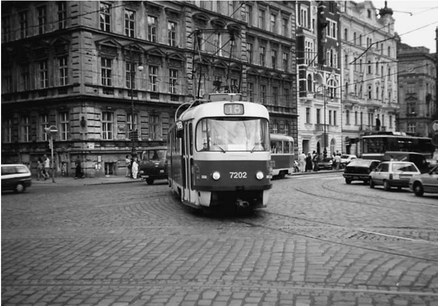
Figure 4.9: Many Tatra Smichov trams remained in operation at the turn of the twenty-first century; the scene here is Prague, near the Tatra factory. Though later models were articulated, with a truck in the middle, Tatra trams had virtually the same control and braking systems as had been devised by Thomas Conway's Presidents' Conference Committee in the early 1930s. (Author's photo)
