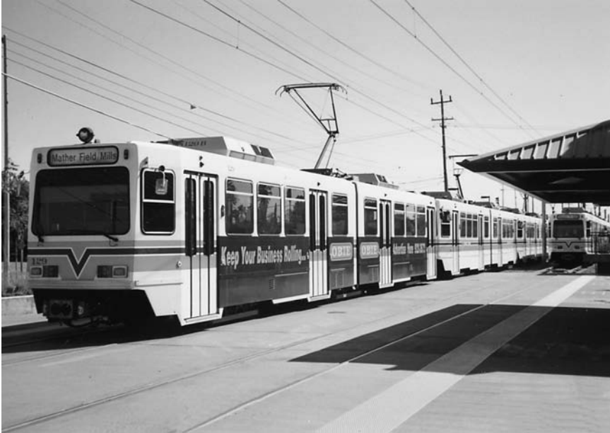
Figure 5.2: In Sacramento, the Regional Transit District's light rail lines largely follow former railroad alignments, as do light rail lines in many other American cities. But in some places, including the vicinity of the state capitol building, Sacramento's LRVs literally become "streetcars." There are several technological distinctions between the newest LRVs and traditional streetcars, however: compact solid-state electrical components take up less space underneath—so cars can therefore have lower floors—and on-board inverters change the direct current (DC) from the overhead wires to 3-phase alternating current (AC). This photo shows another distinction; the cars are articulated, with a truck on each end and another supporting the jointed section in the middle. Passengers validate a ticket inside the car after boarding, a technique borrowed from European practice. (Author's photo)
