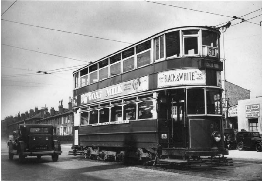
Figure 3.3: A London Transport double-decker, of which there had been thousands in the 1920s, is seen here just a few months before its replacement by trolley buses in 1938; the twin overhead wires are already in place. (Henry Priestly photo, courtesy National Tramway Museum, Crich, Derbyshire)
