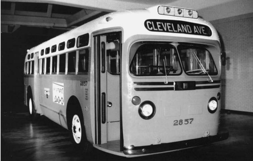
Figure 4.8: The technical data-sheet on this bus reveals that it was built by in 1948 by the GMC Truck and Coach Division, Pontiac, Michigan; designated type TDH (transit, diesel, hydraulic transmission); and delivered to National City Lines of Chicago, then sent to Terre Haute, Indiana, and then in late 1954 to Montgomery, Alabama. There were countless GM TDHs, but none remotely as historic as the 2857 because of what Rosa Parks did when she was told to “move to the back of the bus.” (From the Collections of The Henry Ford, copy and reuse restrictions apply http://www.TheHenryFord.org/copyright.html .)
