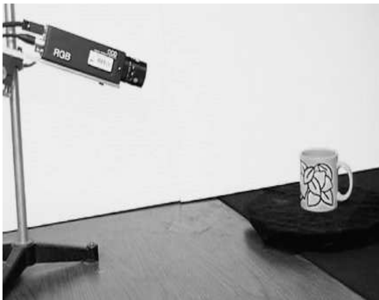
Fig. 11.14. The objects were placed at the center of a motorized turntable. The turntable was rotated through 360 degrees. An image was acquired with a fixed camera at every 5 degrees of rotation. Reprinted with permission from COIL.
