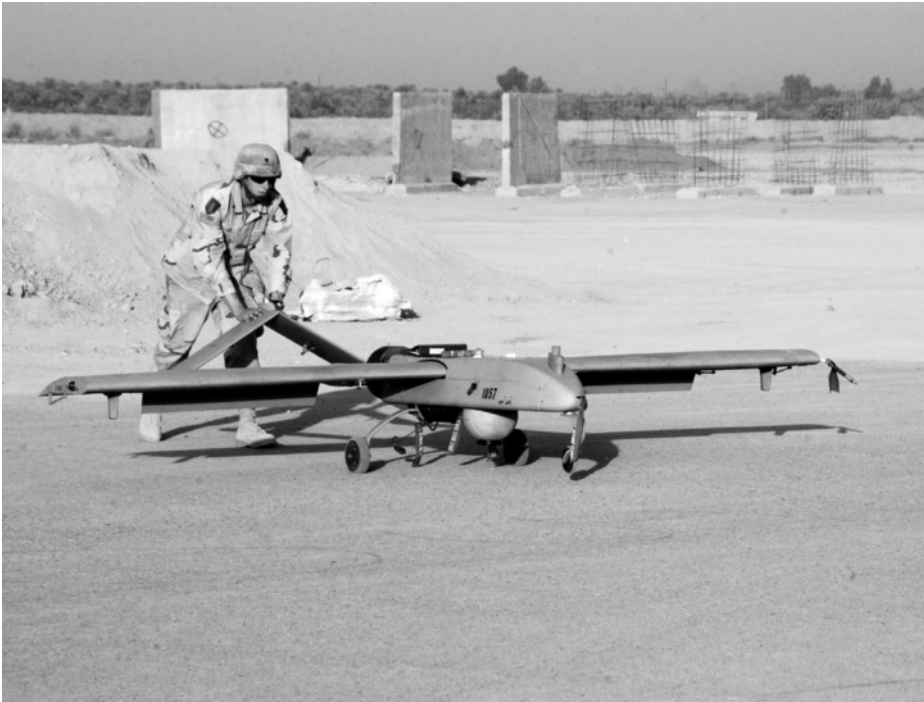
Figure 9-4 A U.S. Army soldier of Company A, 101st Military Intelligence Battalion, 3rd Brigade Combat Team, 1st Infantry Division prepares a Shadow 200 unmanned aerial vehicle (UAV) for launch at Forward Operating Base Warhorse in Iraq (September 24, 2004). Researchers at ARL are studying how to improve human-robot interactions to optimize the performance of robot-soldier teams in future combat environments. (Credit: Photograph courtesy of the U.S. Army.)
