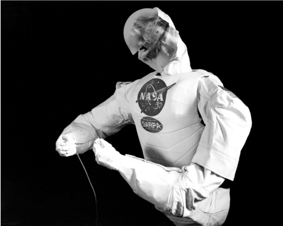
Figure 8-13 Robonaut is a humanoid robot designed by NASA at the Johnson Space Center (JSC) in a collaborative effort with the Defense Advanced Research Projects Agency (DARPA). The Robonaut project seeks to develop and demonstrate a robot system that can function as a human astronaut during extravehicular activity (EVA). This picture shows Robonaut B, the newer of two NASA robots used in hand-in-hand testing with human astronauts. (Credit: Courtesy of NASA/JSC.)
