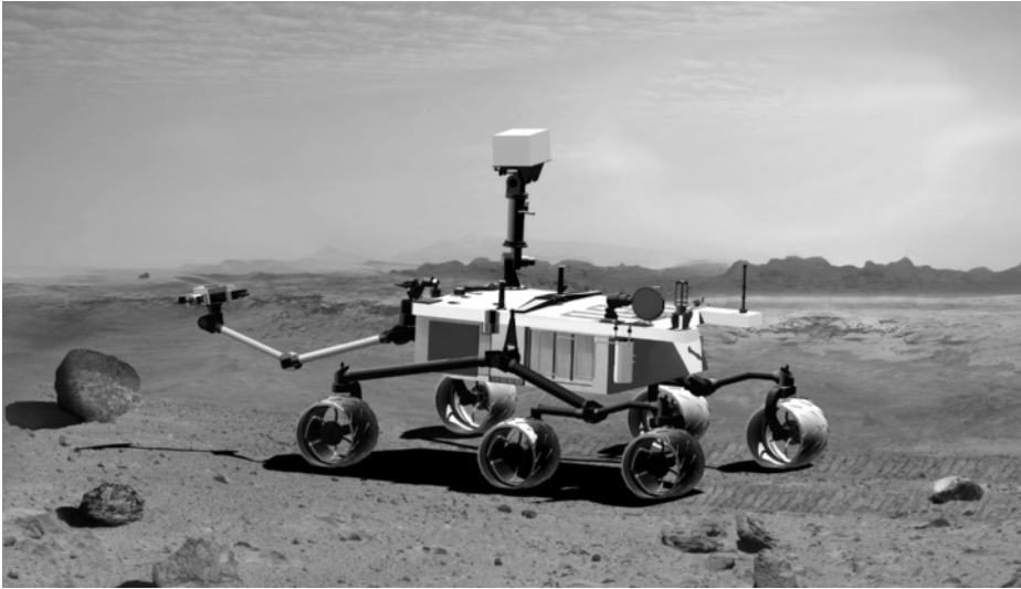
Figure 7-4 This artist's concept shows NASA's planned Mars Science Laboratory (MSL) on the Red Planet (circa 2010) with a robot arm extended to the front of the rover. With a greater range than any previous robot rover used on Mars, the MSL will be able to analyze dozens of samples scooped up from the soil and cored from rocks at scientifically interesting locations on the planet. One of the primary objectives of this sophisticated robot explorer is to investigate the past or present ability of Mars to support life. This artist's rendering shows the MSL. (Credit: Artist's concept courtesy of NASA/JPL-Caltech.)
