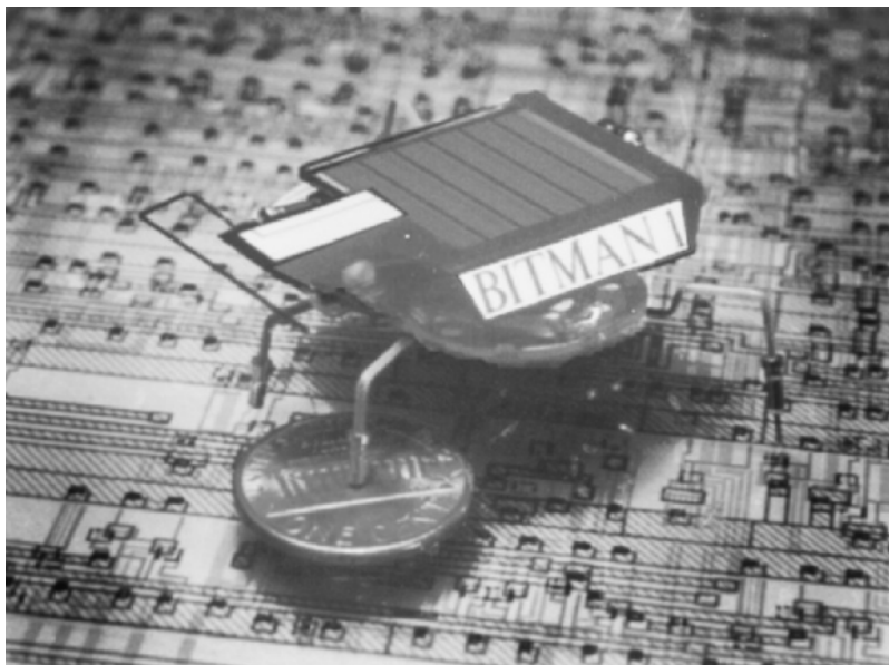
Figure 2-10 A tiny BEAM robot called the Bitman robot. The acronym BEAM stands for biology, electronics, aesthetics, and mechanics. BEAM robots, developed by Los Alamos scientist Mark Tilden, are modeled on the simple, repetitive biological processes of insects. (Credit: Photograph courtesy of the U.S. Department of Energy/Los Alamos National Laboratory.)
