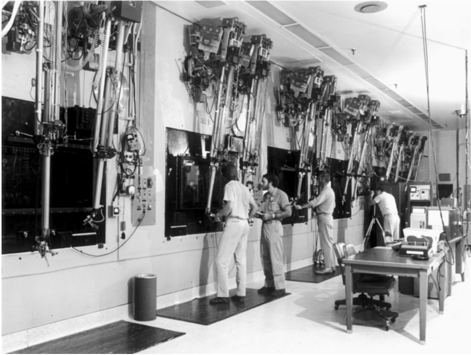
Figure 8-9 These nuclear industry workers are using sophisticated master–slave manipulators to safely handle highly radioactive materials. The technician controls the master manipulator, while on the other side of the shielded wall (which includes special leaded-glass windows) the slave manipulator performs the operations that technician wants to perform involving intensively radioactive materials. This type of hot cell facility is the only practical way that such operations can take occur without exposing the workers to dangerous doses of nuclear radiation. (Credit: Courtesy of the U.S. Department of Energy.)
