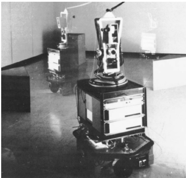
Figure 1-3 The historic picture shows Shakey, the pioneering mobile robot, and a companion robot (in the background) moving through an indoor test range in the late 1960s at SRI (Stanford Research Institute). (Credit: Photograph courtesy of the U.S. Navy/Office of Naval Research.)
