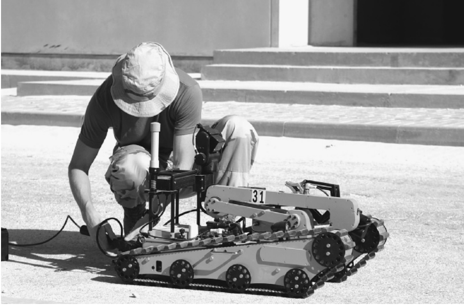
Figure 1-2 A U.S. Navy explosive ordnance disposal (EOD) technician prepares a remotely operated military robot to safely disable an improvised explosive device (IED). This training exercise took place in Southwest Asia on November 10, 2004, in support of Operation Enduring Freedom—the global war on terrorism led by the United States. (Credit: Photograph courtesy of the U.S. Navy.)
