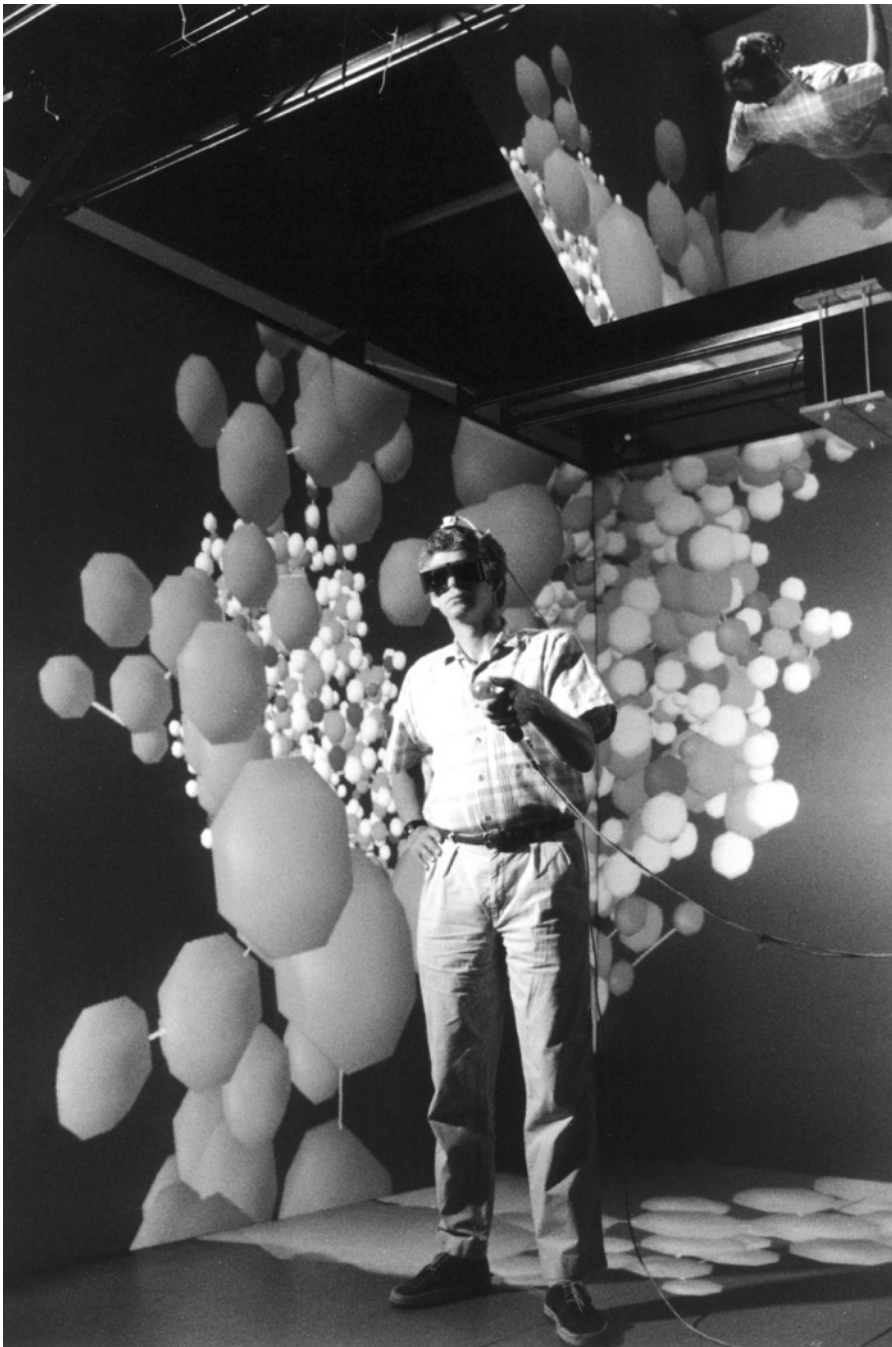
Figure 8-16 A scientist at the Argonne National Laboratory (ANL) uses an automatic virtual reality environment to examine the way complex biological molecules link up and form strings. The scientist can stop the simulation at any point and quite literally move around inside the image to see changes and unique linkages from all angles. This application of virtual reality is a powerful starting point in biomedical research, pharmaceutical development projects, and materials science. (Credit: Image courtesy of U.S. Department of Energy/Argonne National Laboratory.)
