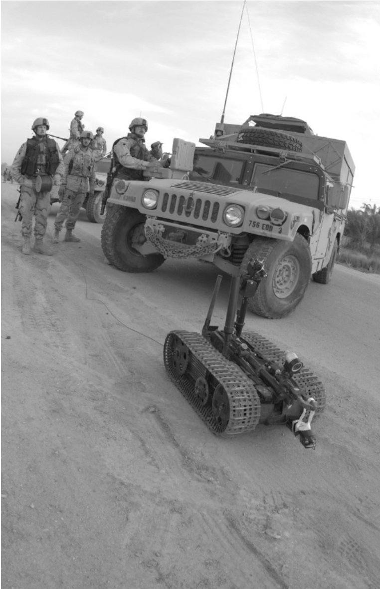
Figure 7-10 A U.S soldier deploys a remotely controlled explosive ordnance disposal (EOD) robot to detonate a possible improvised explosive device (IED) in Al Iskandariyah, Iraq on February 27, 2005. (Credit: Photograph courtesy of the U.S. Army.)
