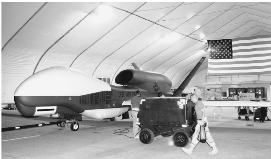
Figure 4-15 The U.S. Air Force's high- altitude, unmanned aerial vehicle (UAV), called Global Hawk, being prepared for a surveillance, and reconnaissance mission at an air base in Southwest Asia (2005). (Credit: Photograph courtesy of the United States Air Force.)
