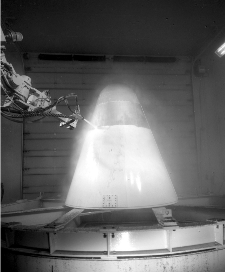
Figure 4-4 The picture (taken April 15, 2004) shows a robotic water-blasting system developed by NASA to automatically remove thermal protection materials and coatings from recovered space flight hardware. During refurbishment operations, the robot system uses a stream of high-pressure water to carefully remove expended thermal protection materials without damaging the underlying structure and without resorting to the use of hazardous chemical strippers. The use of this automated robotic system improves worker safety by reducing human exposure to high-pressure water and high-velocity debris fragments. (Credit: Photograph courtesy of NASA/MSFC.)
