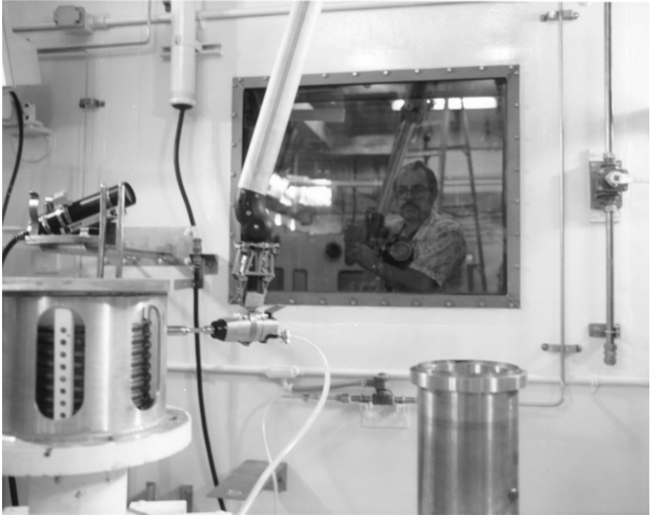
Figure 2-2 Within the American nuclear weapons program, plutonium operations have been conducted in specialized hot cell facilities that protect workers and the surrounding environment. Here, a weapons facility worker (circa 1980) uses a teleoperator to remotely perform complicated mechanical operations on a piece of plutonium-contaminated equipment. Starting with the Manhattan Project, an assortment of ever-more sophisticated robotic devices have allowed nuclear workers to safely and comfortably handle materials that are dangerously radioactive and toxic. (Credit: Photograph courtesy of the U.S. Department of Energy.)
