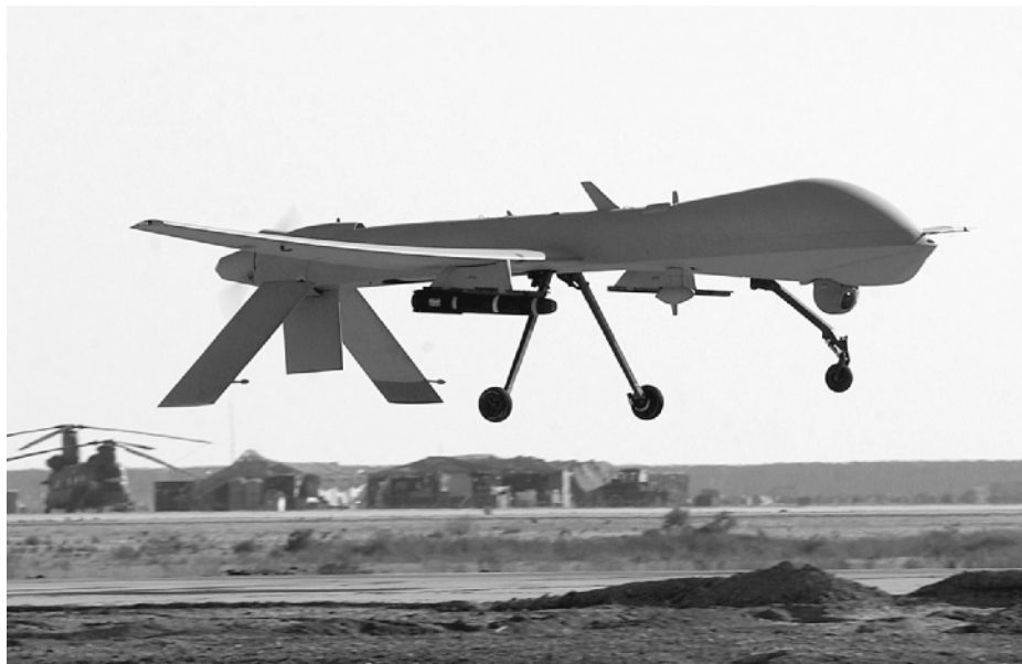
Figure 2-11 This photograph shows a United States Air Force RQ-1 Predator from the 46th Expeditionary Reconnaissance Squadron landing at Tallil Air Base, Iraq. The Predator is a remotely piloted vehicle that provides real-time surveillance imagery in support of Operation Iraqi Freedom. (Credit: U.S. Air Force Photo by Staff Sgt. Suzanne M. Jenkins.)
