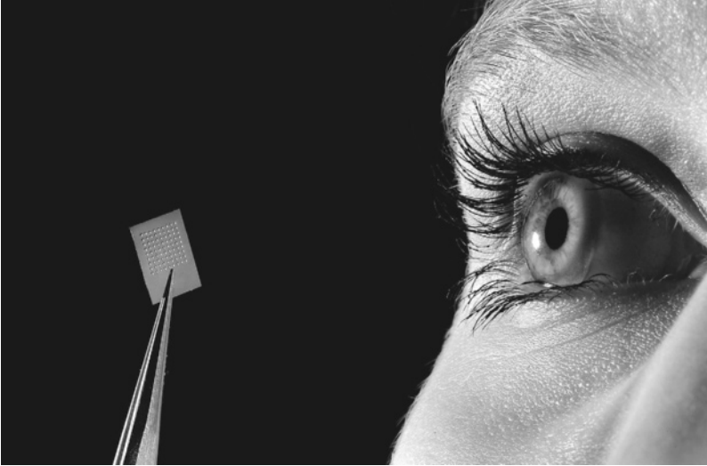
Figure 1-10 This is a prototype of the MEMS-based array that may some day be inserted onto the retina of a blind person to provide some level of useful vision. The prototype microelectromechanical system (MEMS) device was designed by Murat Okandan at Sandia National Laboratories in Albuquerque, New Mexico, under a research grant from the U.S. Department of Energy. (Credit: Photograph courtesy of the U.S. Department of Energy/SNLA).
