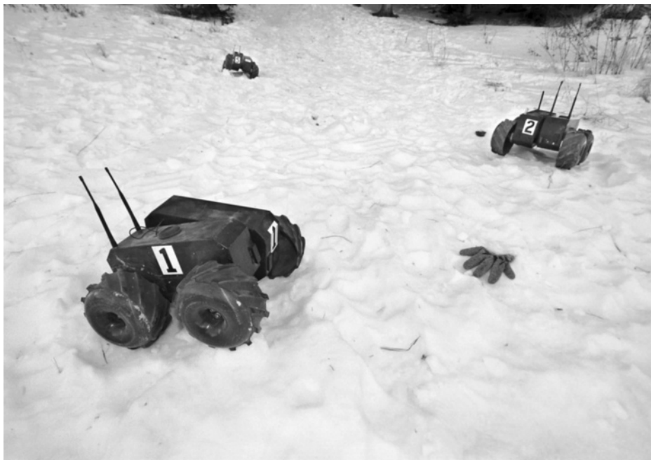
Figure 4-17 This picture shows a team of mini-robots from Sandia National Laboratories demonstrating how the laboratory’s swarm-algorithm-based computer program would help rescuers quickly locate a skier buried under an avalanche. (Credit: Photograph courtesy of U.S. department of Energy/Sandia National Laboratories.)
