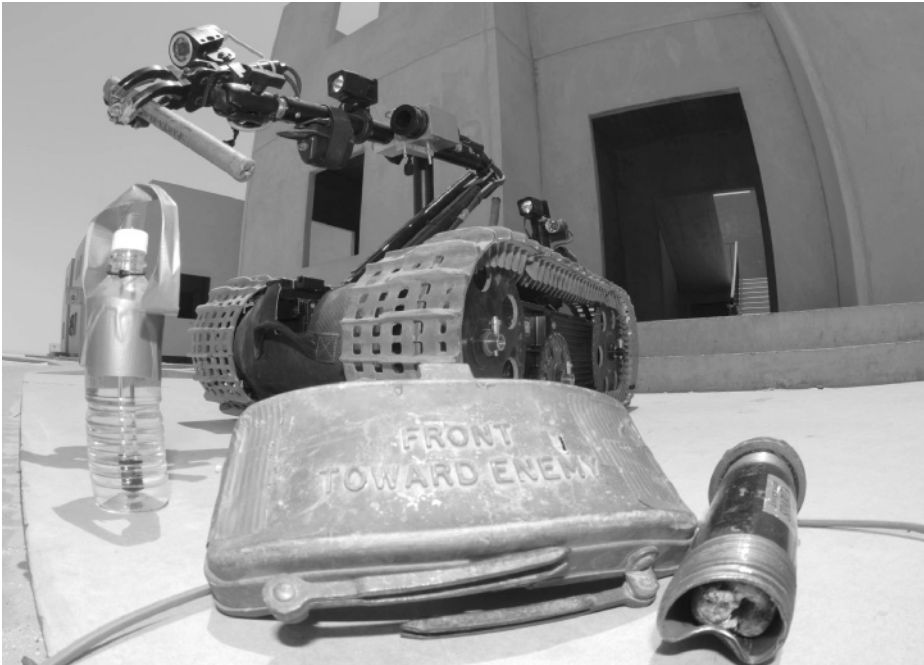
Figure 5-8 This photograph shows a Talon 3B robot as it recovers a stick of dynamite and other explosive devices at a military training range in Bahrain, Persian Gulf. The explosive devices used in this training exercise (June 2005) are commonly seen by American military personnel deployed in Iraq. Explosive ordnance disposal (EOD) technicians operate the robot from safe locations through the use of monitors and video equipment attached to the unit. The robot is designed for the search and destruction of improvised explosive devices (IEDs), as well as other forms of ordnance found in Iraq. (Credit: Photograph courtesy of the U.S. Navy.)
