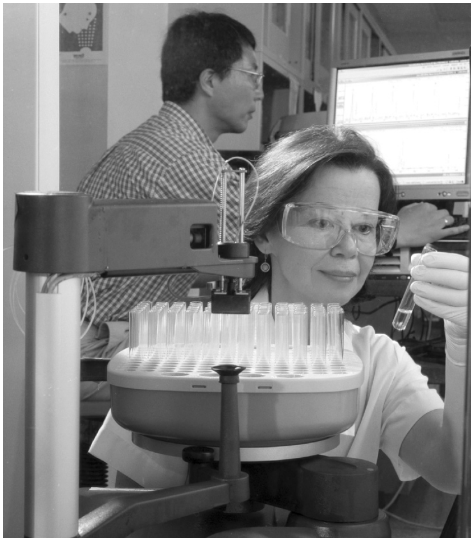
Figure 9-3 Argonne National Laboratory (ANL) scientists work with the first robot of its type in the United States to automate protein purification. The robot, which is housed in a refrigerator, is an integral part of the Argonne-based Midwest Structural Genomics Center's plan to automate the protein crystallography process. The ANL robotic system can purify six proteins per day versus previous procedures that required two to three days per protein. (July 2004) (Credit: Photograph courtesy of the U.S. DOE and Argonne National Laboratory.)
