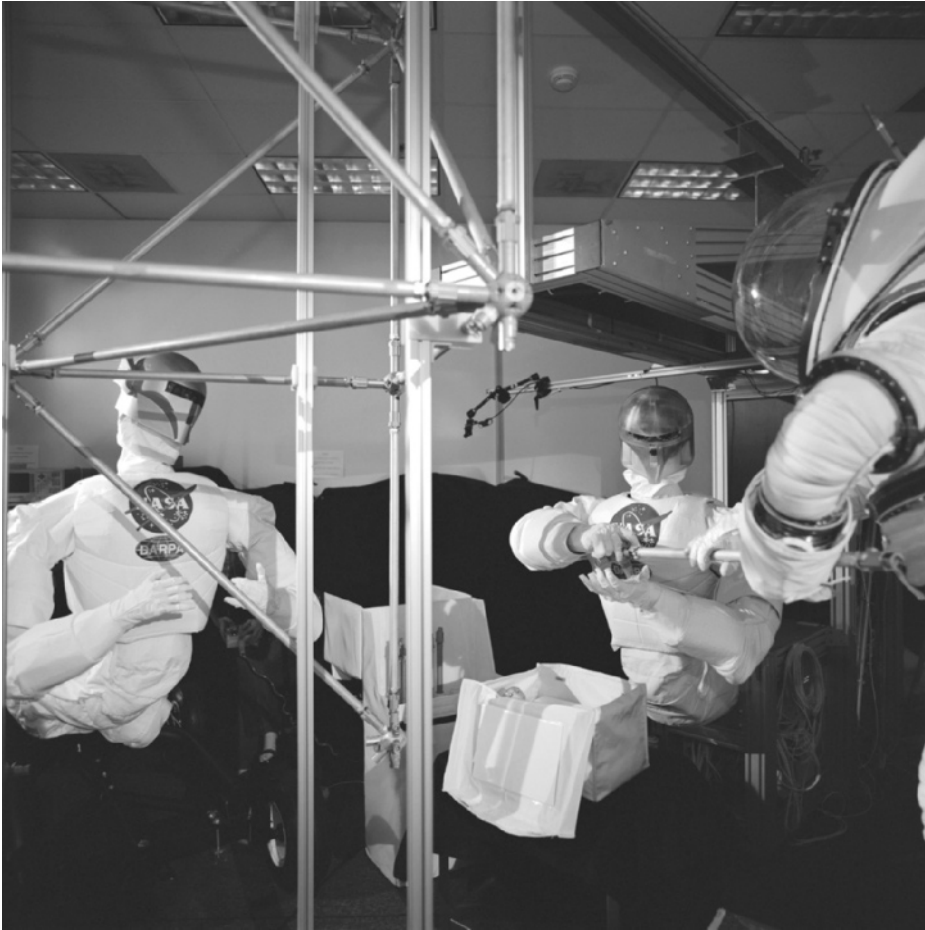
Figure 7-5 A space-suited human astronaut (on right) practices an assembly and construction task together with two Robonauts (humanoid robots), during a simulated extravehicular activity at the Johnson Space Center in 2003. Second- and third-generation designs of such humanoid robots would serve as valuable machine partners, helping human beings permanently settle the Moon and (later) explore Mars. (Credit: Photograph courtesy of the NASA/Johnson Space Center.)
