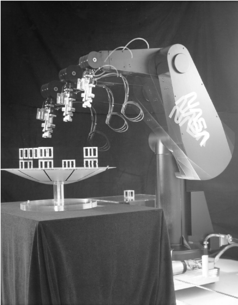
Figure 2-8 This photograph shows a sequenced series of actions by a PUMA robotic arm during studies (circa 1989–1990) at the NASA Ames Research Center in Mountain View, California. (Credit: Photograph courtesy of NASA/Ames Research Center.)
