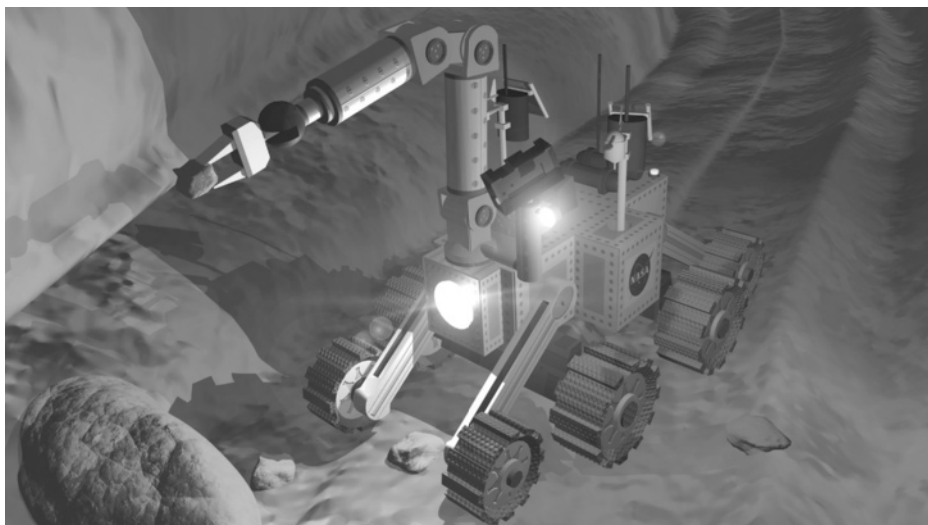
Figure 7-1 This is an artist's concept of an advanced, semi-autonomous robot rover making remote sample collections at the Moon's south pole. With minimal supervision and teleoperation by controllers on Earth, this type of advanced robot sample collector would help validate the presence of water ice and quantify any promising resource data collected by lunar-orbiting resource reconnaissance spacecraft. The presence of ample quantities of water ice in the permanently shadowed polar regions of the Moon would be a major stimulus in the development of permanent human bases. Robot-assisted lunar ice mining could become the major industry on the Moon later this century. (Credit: Artist's concept courtesy of NASA/Johnson Space Center.)
