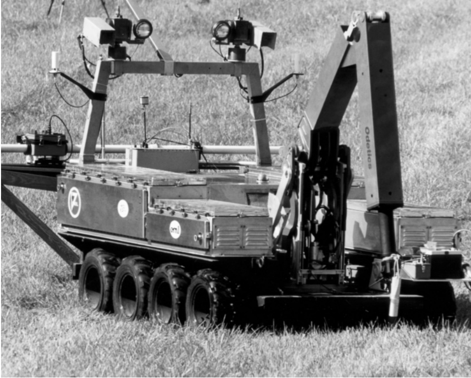
Figure 5-10 The picture provides a close-up view of a remotely operated field robot (built circa 1990) at the Oak Ridge National Laboratory (ORNL). The mobile nuclear robot is equipped with electronic systems, sensors, and computers. Designed to perform outdoor surveys of radioactive waste storage sites, the diesel-engine powered, eight-wheeled, all-terrain vehicle is driven across the field being inspected by a human teleoperator, who remains comfortably and safely seated at a remote control console. (Credit: Photograph courtesy of Department of Energy/Oak Ridge National Laboratory.)
