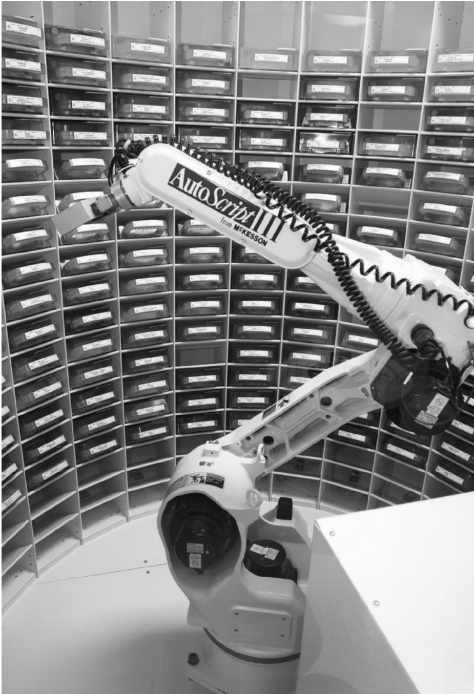
Figure 5-1 This picture shows the Autoscript III, a prescription filling robot at the National Naval Medical Center in Bethesda, Maryland, as it picks up a properly-coded bin of medication. The modified robot is one of two used in the hospital pharmacy. (Credit: Photograph courtesy of the U.S. Navy.)
