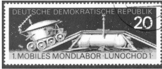
Figure 2-6 This 1971 postage stamp from the former German Democratic Republic (East Germany) depicts the Soviet Lunokhod 1 robot rover departing the lander spacecraft. During the Soviet Luna 17 mission to the Moon in 1970, the mother spacecraft soft-landed on the lunar surface in the Sea of Rains and deployed the Lunokhod 1 robot rover vehicle. Controlled from Earth by radio signals, the eight-wheeled mobile robot traveled for months across the lunar surface, transmitting more than 20,000 television images of the Moon's surface and performing more than 500 soil tests at various locations. (Credit: Photograph courtesy of author.)
