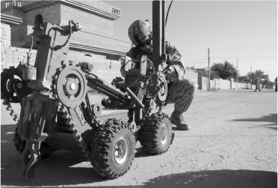
Figure 6-2 At Camp Fallujah, Iraq (November 27, 2005), a U.S. Marine Corps explosive ordnance disposal (EOD) technician prepares to deploy a remotely operated vehicle (ROV) to neutralize a buried improvised explosive device (IED). The suspected IED was buried in a dirt mound on the side of the road next to an old IED crater. (Credit: Photograph courtesy of the U.S. Marine Corps.)
