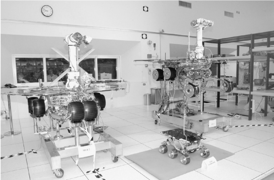
Figure 4-10 Prior to launch, the twin Mars Exploration Rovers (MERs), Spirit (elevated on right) and Opportunity (elevated on left) pose with the flight spare of their ground-breaking robot predecessor, the Mars Pathfinder minirover (on floor) at NASA's Jet Propulsion Laboratory in February 2003. (Credit: Photograph courtesy of NASA/JPL.)
