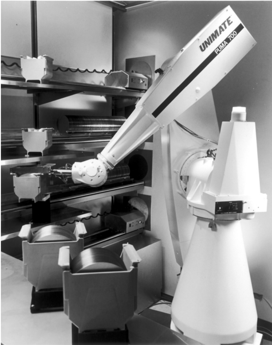
Figure 4-3 This photograph shows a Unimate PUMA 700 robot. The versatile pick-and-place industrial robot was designed (in the 1980s) to perform a variety of tasks in assembly, material handling and transfer, joining, inspection, and palletizing. (Credit: Photograph courtesy of Unimation Incorporated, a Westinghouse Company.)
