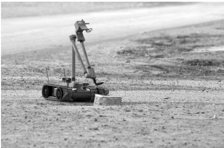
Figure 8-3 A U.S. Army explosive ordnance disposal (EOD) robot, called i-Robot, pulls the wire of an alleged improvised explosive device (IED) found by Iraqi police on November 3, 2004. The EOD robot (shown here) was operated by a team of American soldiers, who examined the suspicious device from a safe distance, using the robot's two on-board cameras and mechanical arm. In this instance, the suspicious device proved to be a decoy, set in place by terrorists to harass Iraqi policemen and the U.S. soldiers assisting them. (Credit: U.S. Navy New Photo.)
