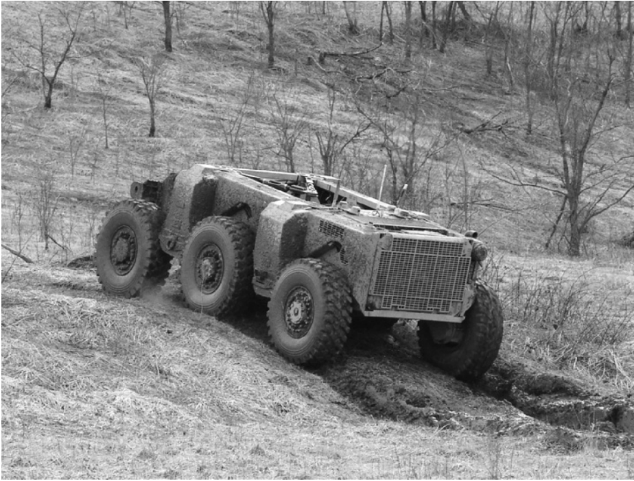
Figure 9-5 On April 28, 2006, DARPA and the U.S. Army unveiled the Crusher unmanned ground combat vehicle. Crusher is a six-wheeled, all-wheel drive, hybrid electric, skid-steered unmanned ground combat vehicle (UGCV). The robot vehicle is being equipped with state-of-the-art perception capabilities, and will be used to validate the key technologies necessary for future UGCVs to perform military missions autonomously. The National Robotics Engineering Center (NREC) at Carnegie Mellon University in Pittsburgh, Pennsylvania, is the prime contractor for Crusher. (Credit: Photograph courtesy of the U.S. Army.)
