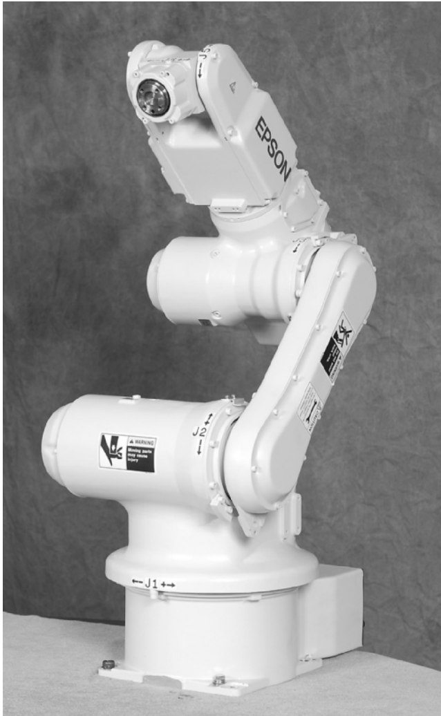
Figure 4-1 This is the EPSON Pro Six Model PS5DSC robot—an example of a computer-controlled, modern industrial robot with electric motors and six degrees of freedom. (Credit: Photograph courtesy of EPSON Robots.)
