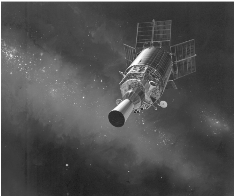
Figure 5-5 This artist's rendering shows a U.S. Air Force Defense Support Program (DSP) satellite in its role as a robotic orbiting sentry. Since 1970, these surveillance satellites have played a vital role in the defense of the United States by detecting and reporting missile launches. (Credit: Artist rendering courtesy of the U.S. Air Force and Northrop Grumman.)
