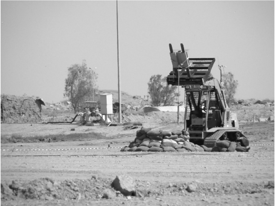
Figure 9-2 During Operation Iraqi Freedom (OIF) robots from the Air Force Research Laboratory (AFRL) helped to counter bomb threats. This photograph shows an all-purpose remote transport system (ARTS) clearing an area at Balad Air Base, Iraq, of unexploded ordnance (UXO). Airmen responsible for explosive ordnance disposal (EOD) activities use such remotely operated systems to safely and effectively clear important ranges, while staying out of harm's way. (Credit: Photograph courtesy of U.S. Air Force.)
