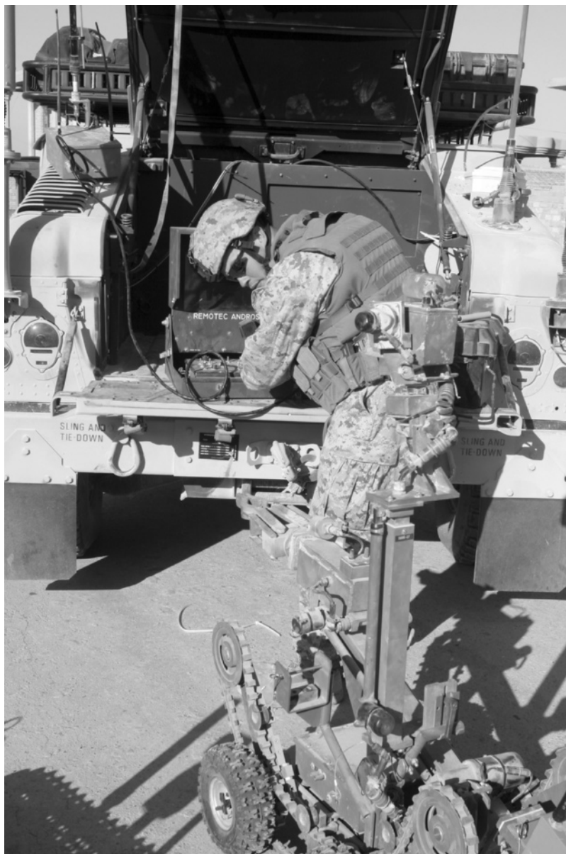
Figure 5-7 A U.S. Marine Corps explosive ordnance disposal (EOD) technician prepares to deploy a remotely operated robot vehicle to detonate a buried improvised explosive device (IED) near Camp Fallujah in Iraq (November 27, 2005). The suspected IED was buried in a dirt mound on the side of the road next to an old IED crater. (Credit: Photograph courtesy of the U.S. Marine Corps.)
