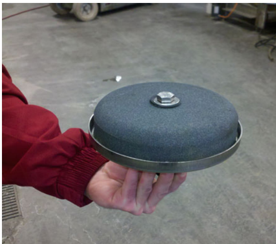
Fig. 12 Photo of one of the porous diffusers
