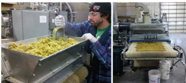
Fig. 16 Cellencor microwave dryer showing details of feeding the fungal biomass and the dried product emerging from the drying tunnel
