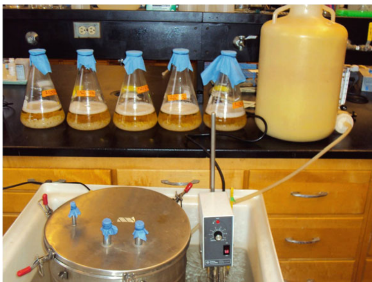
Fig. 13 Pre-culturing set-up for preparing pilot plant inoculum
