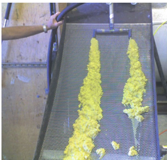
Fig. 15 Secondary screen dewatering equipment
