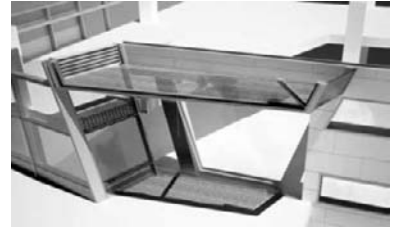
Fig. 11-13 At Great Ormond Street Childrens' Hospital our brief was to create a folded glass wall design including final construction details. An original wireframe model for the building was provided and input to a parametric model. Architect: Llewelyn Davies Yeang
