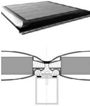
Fig. 9 Example of a film based vacuum insulation pane, consisting of a fumed silica core which tightly sealed into a high barrier envelope of a three-layer metallized polymer film after evacuation.
