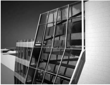
Fig. 17-19 A new building for Great Ormond Street Hospital in London, approaching the construction phase, uses a double façade where expelled air from the building is passed between the outer walls to reduce the need for mechanical ventilation in the building. The outer glass expresses the direction of air movement in the thermal flue behind. Architect: Llewelyn Davies Yeang
