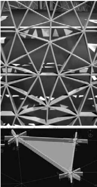
Fig. 1-3 Above and below: This project for a tower in Russia, currently completing the detailed design stage, has a cladding design developed as a mathematical model from which we generated engineering data that allowed us to modify the design to optimise shading created by the geometry of the framing.
