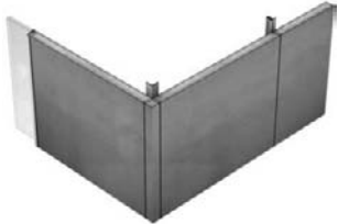
Fig. 3 In the detached government-subsidized housing, the sandwich panels form a part of the main load-bearing construction; the panels are only connected by slender angle sections
