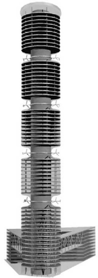
Fig 2: Wind energy applied in a high rise building (concept Bouke Braun under supervision of, among others wind expert Dr. Ir. Sander Mertens). The design is part of a research on the feasibility of wind energy in high rise buildings. The research was carried out on basis of a location in Rotterdam (in the coastal area of the Netherlands). The warpage concept with a rotating ring is designed such that the turbines are always oriented directly into the wind. Due to the shape of the building the wind velocity in the necking-areas in is considerably higher.
