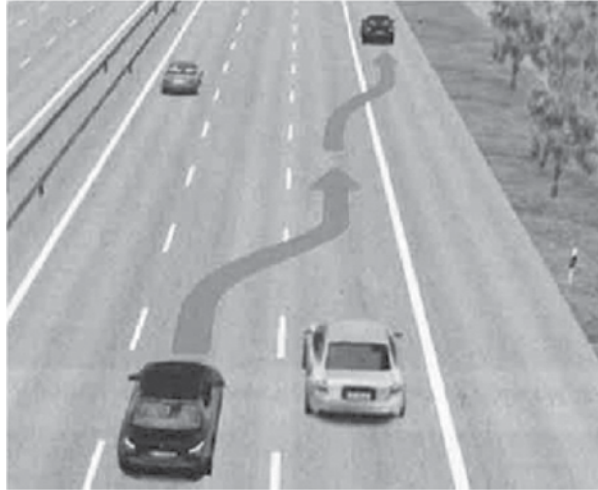
Figure 11.2 Level 4 automation concept to bring a vehicle to a safe stop on the shoulder of a highway. (From M. van Schijndel-de Nooij et al. Definition of Necessary Vehicle and Infrastructure Systems for Automated Driving , European Commission SMART 2010/0064 Study Report, Brussels, BE, June 2011, Version 1.2.)
