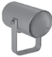
ASIM 334 24 GHz Doppler sensor. Detects vehicles moving into or through its field of view out to 45 m ( \approx 150 ft). Minimum detectable speed: 4 or 8 km/h (2.5 or 5 mi/h). Applications include direction-selective detection and green phase request and extension. (Photograph courtesy of ASIM Xtralis Technologies, Kiel, DE)
