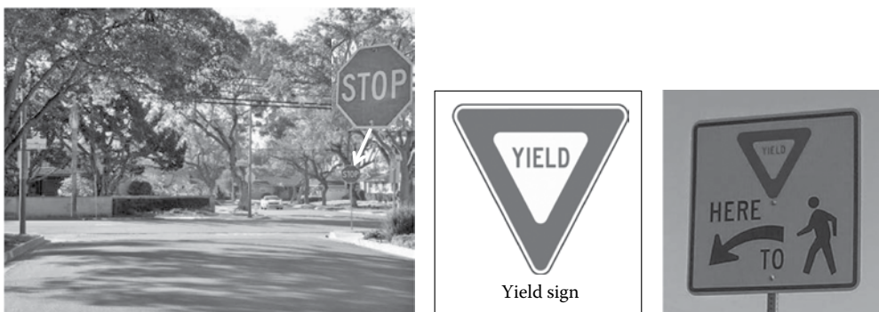
Figure 1.3 Stop sign and yield sign configurations. In the photograph on the left, the stop sign inset shows the octagonal shape of the sign.
