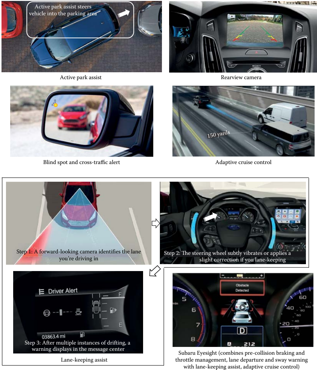
Figure 11.8 Driver assist and crash avoidance features found in vehicles. (Photographs reprinted with permission of Ford Motor Company and Subaru of America.)
