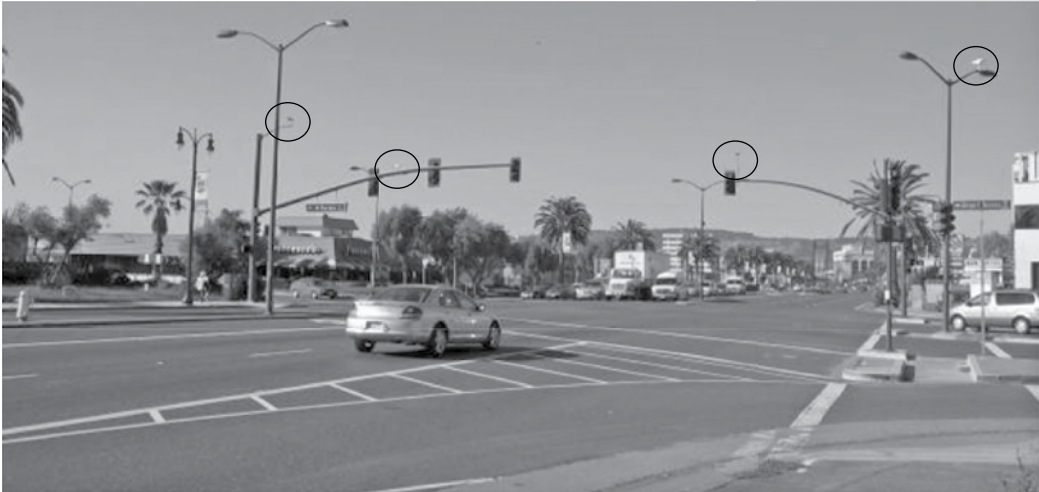
Figure 5.16 VDS camera mounting options include luminaire or signal mast arm mounting. (From LAK.)
