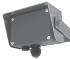
ADEC TDD1 24 GHz Doppler series sensor. Detects vehicles moving through its field of view up to 75 m ( \approx 250 ft). Minimum detectable speed: 4 or 8 km/h (2.5 or 5 mi/h). Applications include direction-selective detection and green phase request and extension. (Photograph courtesy of ADEC Technologies, Eschenbach, CH)
