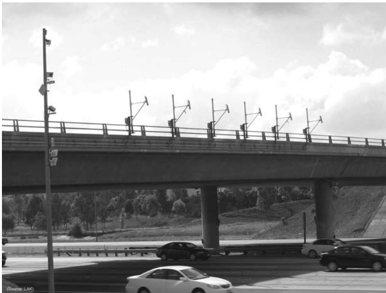
Figure 9.1 Over-lane video cameras and roadside sensor-mounting pole at I-405 V 2 DVS sensor evaluation location.
