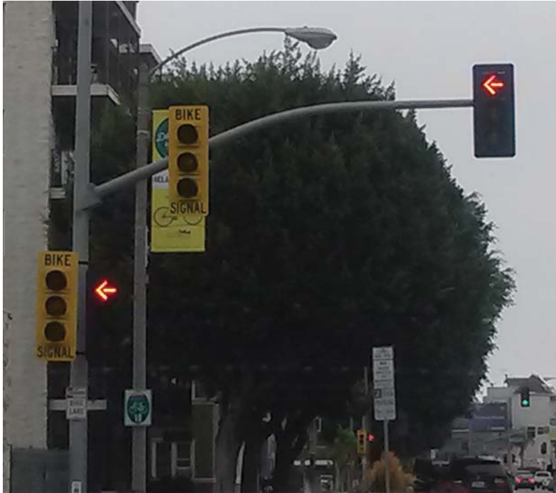
Figure 3.2 Separate traffic signals indicate bicycle right-of-way. (From LAK.)
