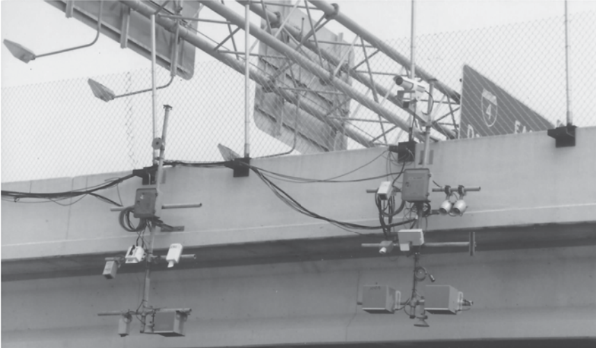
Figure 8.8 Sensors mounted on SR-436 overpass above I-4 at Altamonte Springs evaluation site.
