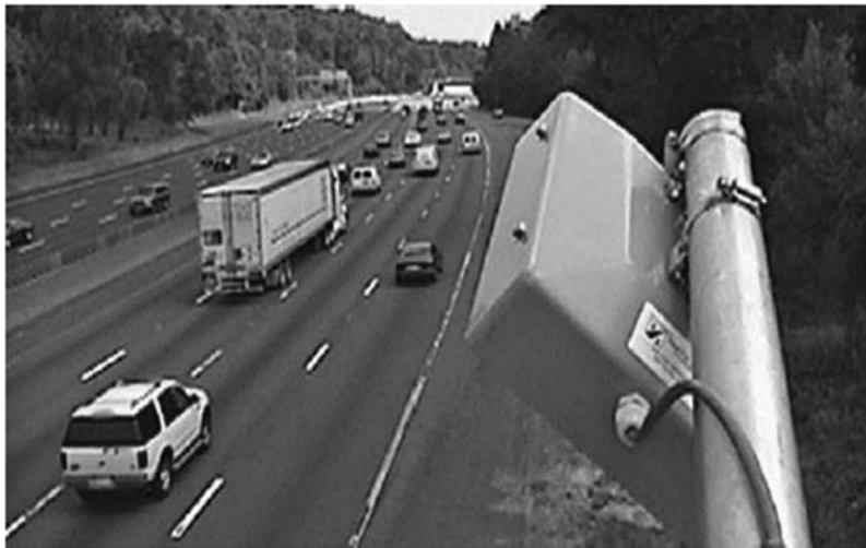
Figure 5.29 SAS-I passive acoustic sensor. (Photograph courtesy of SmarTek Systems, Inc., Woodbridge, VA.)
