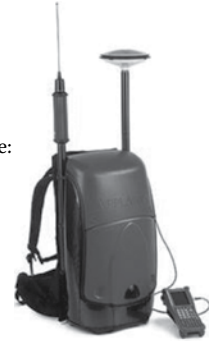
Figure 10.7 GPS-only and combined GPS-INS devices used in University of Washington tests. (Photographs courtesy of Trimble.)
