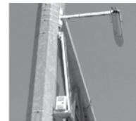
ITMS-100. Solar-powered multi-lane sensor provides vehicle count, speed, and classification by lane. Also road surface temperature for determining snow and ice conditions. Range up to 250 ft (76 m).
