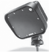
AGD Model 318 FMCW, 24 GHz radar. Speed measurement from 4 km/h to 300 km/h across multiple lanes. Vehicle range measurement from 6 – 150 m. Typical applications include: multi-lane highway vehicle detection, single lane detection for traffic control, dual line detection for rail, wrong-direction detection for highways, sign activation. (Photograph courtesy of AGD, Gloucestershire, UK)
