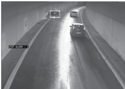
Trafficon-Stopped vehicle in Leutenbach Tunnel, Germany https://www.youtube.com/watch?v=AvjAoJ1EeN4
