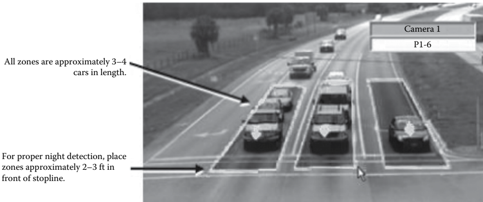
Figure 7.7 Guidelines for placing presence detectors at a stopline for a VideoTrak-IQ™ VDS. (Photograph courtesy of Peek Traffic, Palmetto, FL.)
