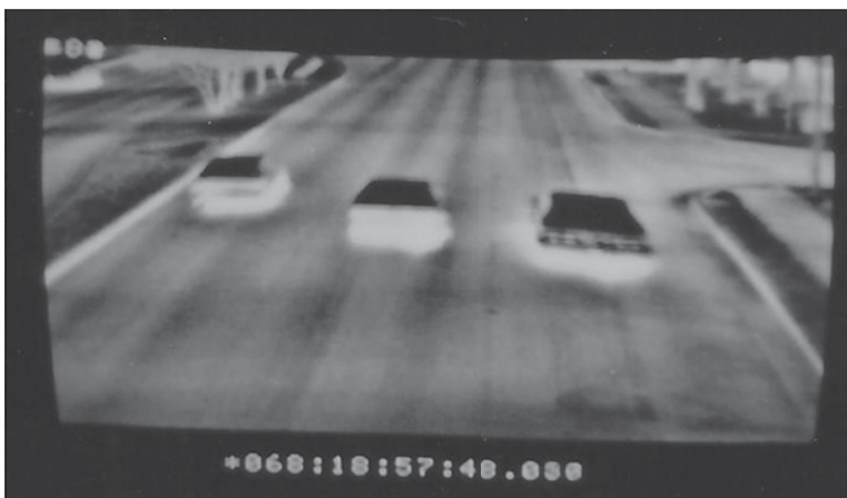
Figure 8.24 Thermal images of vehicles on Oracle Road obtained with the imaging infrared camera system.
