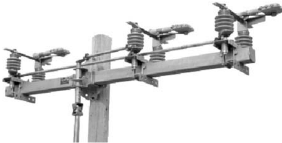
FIGURE 4.19 Typical side break switch disconnector showing operation rod and arc breaking chambers (Hubbell Power System Inc. Type AR, 15 kV 900 A continuous/interruption rating).
