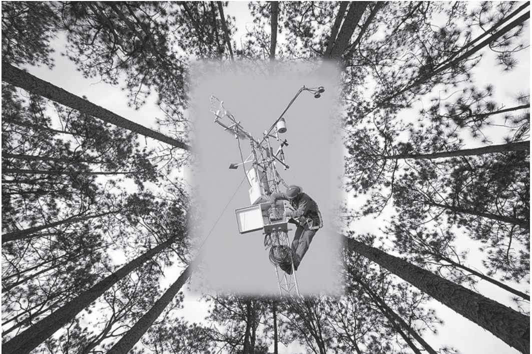
FIGURE 7.10 An eddy-flux tower at the Joseph W. Jones Ecological Research Center at Ichauway, used in measuring carbon and water budgets of longleaf pine ecosystems.
