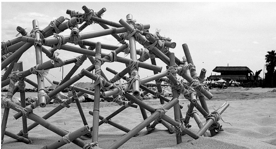
Fig. 4. Reciprocal model of the icosahedron Alt 2v in bamboo, built on sand
