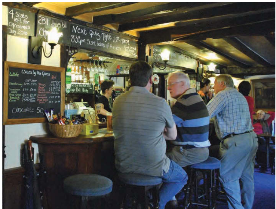
Plate 13 Bare CFLs protruding from luminaires produce unwelcome glare
