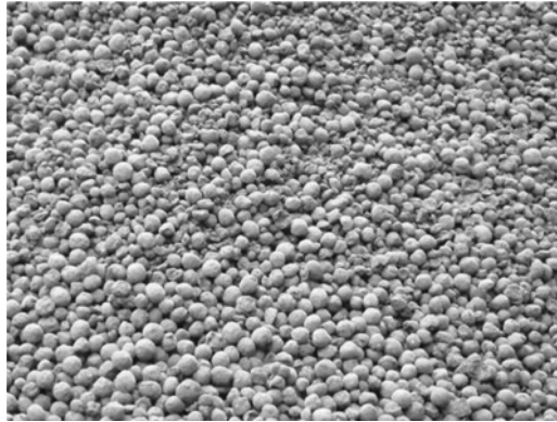
Figure 2.8 Dried sludge from the drying unit of Thessaloniki (Greece) wastewater treatment plant.
