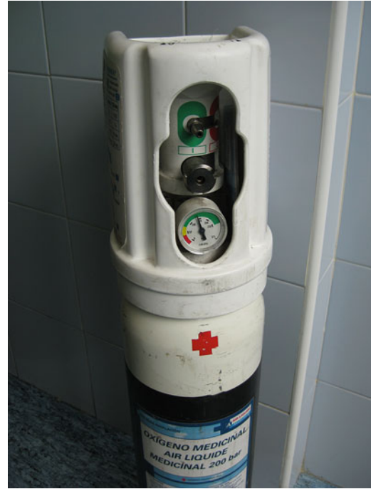
Figure 13.6. Small transportable oxygen tank with protected low-flow regulator. The oxygen inside this tank is pressurized to 200 bar but its outlet is regulated to no more than 3 bar.
