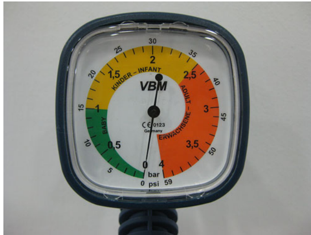
Figure 13.13. Manometer with different recommended driving pressures that can be set according to the age or size of the patient.
