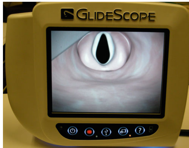
Figure 6.12. The AVL monitor has several buttons along the bottom. From left to right, these are the On/Off, Recording On/Off, transfer file/files to USB port on the right side of the monitor, port image to an external display using the rear video output (HDMI) port, an on-board video tutorial, and a charging indicator. The monitor is displaying an image from the audio-visual tutorial. Recordings are stored on-board and time stamped.
