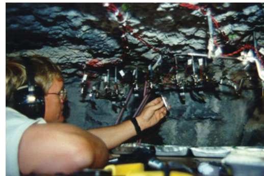
Figure 14.4 Top: Schematic of Hell's Half Acre 1-m infiltration test showing open-bottomed container affixed to an exposed fracture that penetrates an overhanging basalt ledge. Beneath the ledge are drip detectors and collection vessels. Bottom: A worker making adjustments to piezoelectric strips used for monitoring drips. The grid of metal pans is shown in the background, which collected water for determining the spatial distribution of water mass exiting the lower fracture.
