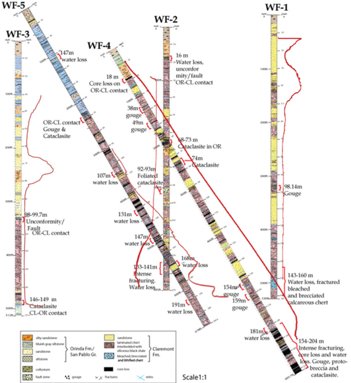
Figure 3.4 Core logs of WF-1~WF-5 boreholes shown in 2D. Note that there is little borehole to borehole correlation. Black colors indicate core loss sections. Superimposed are the FFEC log results in red curves along the boreholes.
