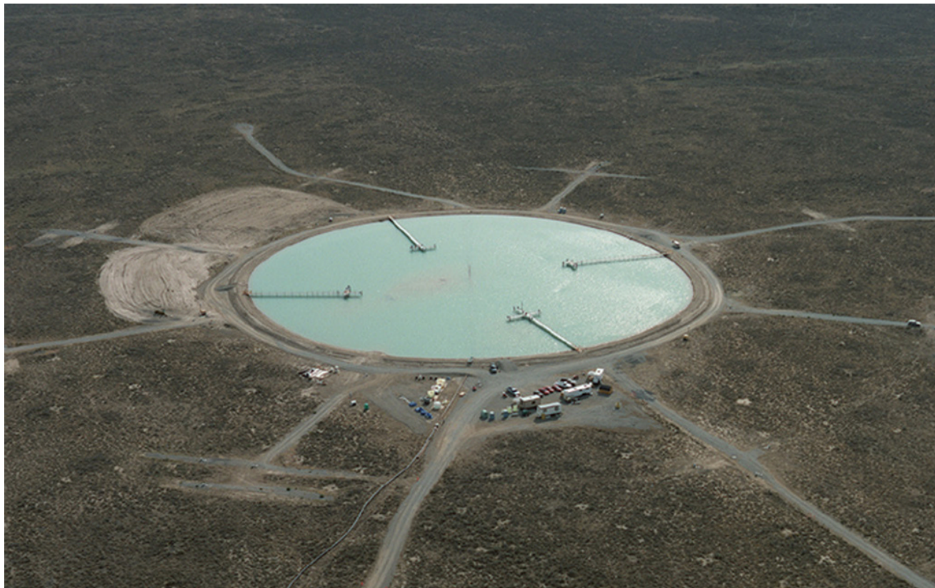
Figure 14.2 Aerial view of the aquifer pumping and infiltration test site. The basin is shown full of water just after tracers were added. Four docks extend out into the basin for access to nested wells and lysimeters. Radial lines are roads to wells at various offsets from the basin. The diameter of the basins is 182 m; for scale, several vehicles can be seen to the left of center.
