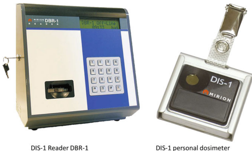
Fig. 5.12 DIS-1 personal dosimeter and reader (Photos courtesy of Mirion Technologies)
