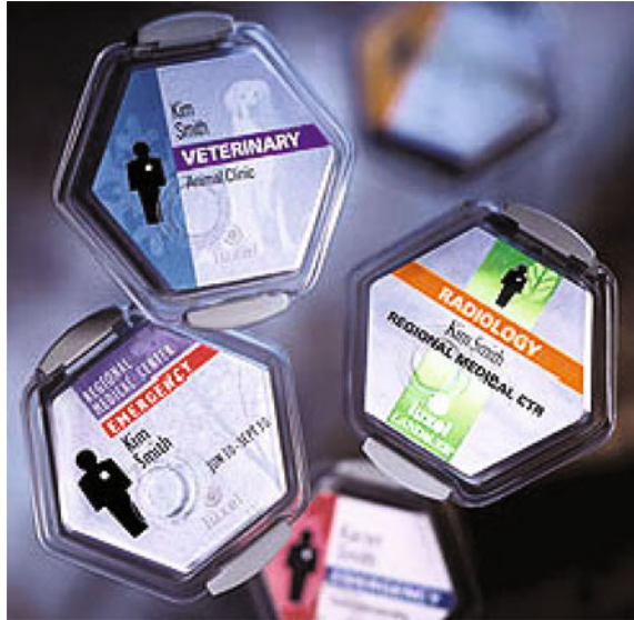
Fig. 5.10 Landauer Luxel® radiation monitoring badge [“Reprinted from monitoring of radiation exposure at https://www.uic.edu/depts/envh/RSS/Badges.html with permission of Landauer, Inc.”]
