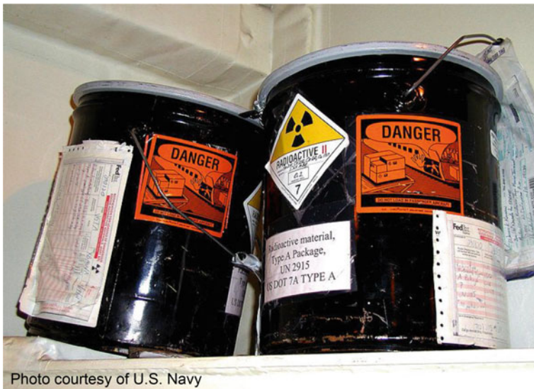
Fig. 15.4 A labeled Type A container with radioactive material
