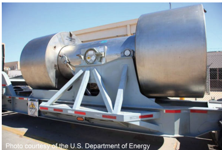
Fig. 15.1 RH- 72-B transuranic waste transportation container
