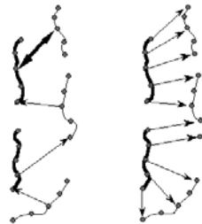
Fig. 8. Matched linked sets. A chain of curve matches is established (left) and all the points in each set are allowed to match as one structure to give uniform closest points (right)
