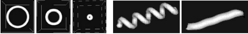
Fig. 3. Evolving curves under mean curvature flow. The first three images show a circle shrinking to a point, and the last two images show a helix shrinking to its axis
