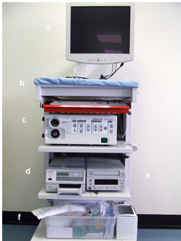
FIGURE 3.1 Typical bronchoscopy stack with (a) high resolution screen, (b) clean surface for bronchoscope and further instruments, (c) light source, (d) printer, (e) DVD burner, (f) storage space for ancillary equipment
