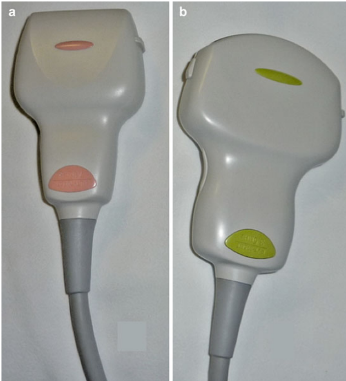
FIGURE 16.1 Commonly used ultrasound probes ( a ) Linear 7–12 MHz probe; ( b ) 3.5–5 MHz curvilinear probe
