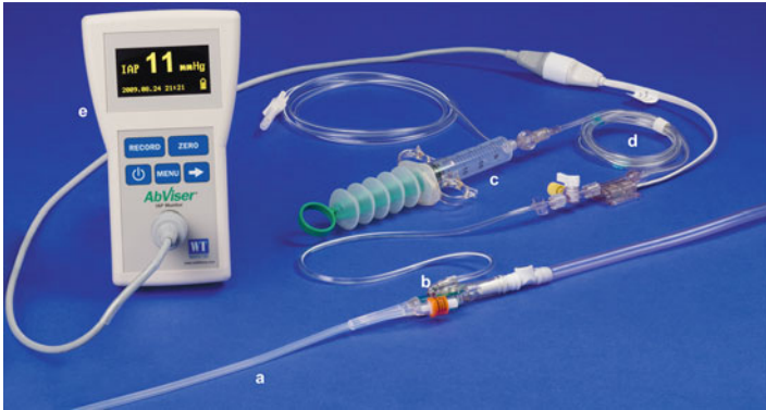
FIGURE 15.1 Equipment to measure intraabdominal pressure: (a) urinary catheter with; (b) side port for injection; (c) syringe attached to three-way-taps; (d) monitoring line with pressure transducer; (e) IAP pressure monitor (Reproduced with kind permission from Wolfe Tory Medical)
