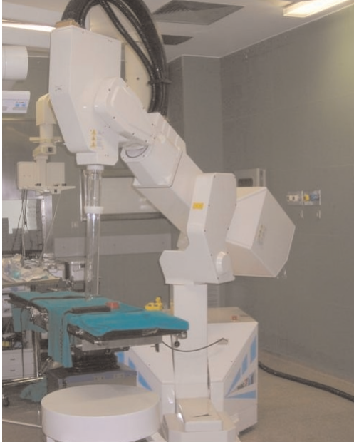
Fig. 5.1 Novac 7 mobile linear accelerator
