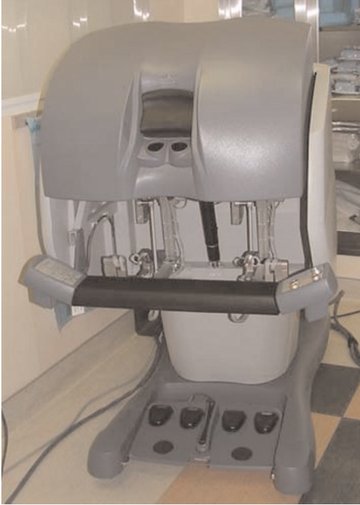
Fig.7.1 Operator console (dimensions 166x97x158 cm, weight 227 kg)
