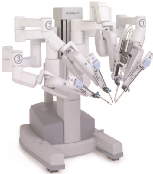
Fig. 7.2 Robotic arms (dimensions 198x94x97 cm, weight 544 kg)
