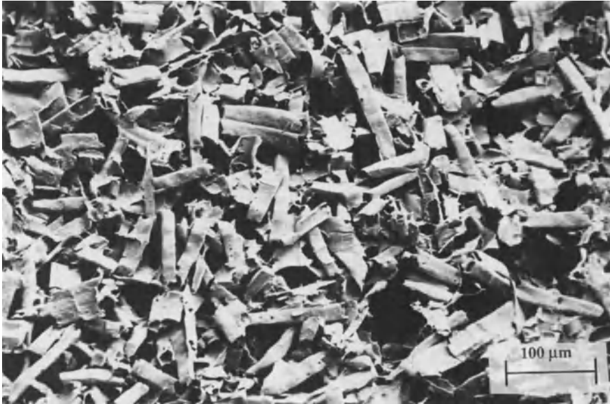
Fig. 2.3. Ray cells from Norway spruce ( Picea abies ) isolated from disintegrated wood material. Scanning electron micrograph
