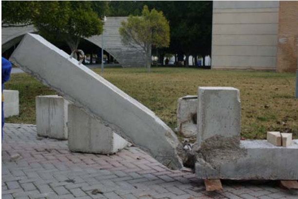
Figure 8: Photograph of the ultimate rupture of prototype 4.
