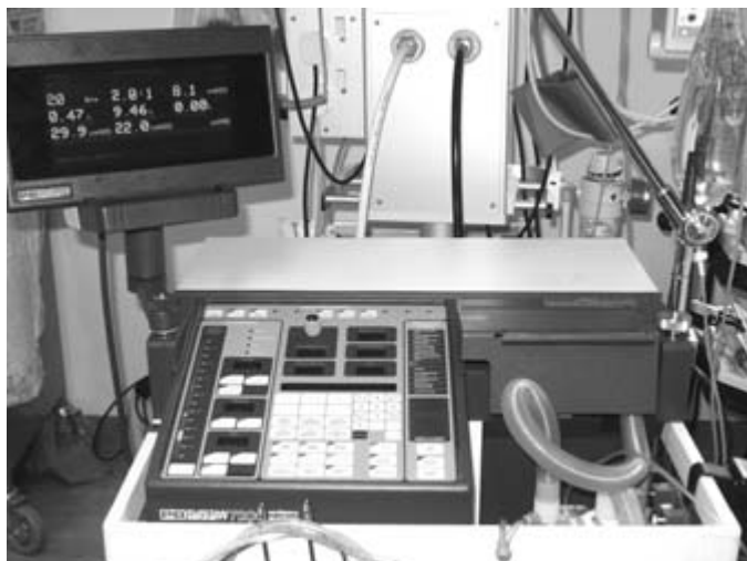
Figure 5.5 ICU ventilator. Soft keys allow control of ventilator settings with display of volumes and pressures generated.
