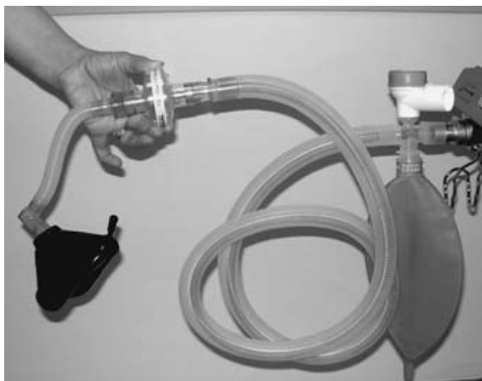
Figure 2.13 The component parts of a breathing system and photograph of the system connected to the common gas outlet on the anaesthetic machine. Note the port on the expiratory valve (white) to allow connection to the anaesthetic gas scavenging system.
